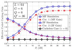
Fig. 3: Effective coded caching gain versus  $P_t$ .
