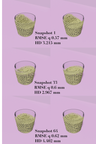
Figure 4: Comparison of the reconstruction of the integration provided by the SPNN (right) with the ground truth (left). The selected snapshots correspond to peaks of the sloshing dynamics of glycerine. Specifically, we present the comparison for snapshots 1, 33, and 64 of the collection. The height of the cup is 7\text{cm} , and it is filled up to 5.6\text{cm} approximately.
