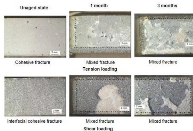
Fig. 1 - Failure surfaces of the Arcan specimen before and after ageing in seawater [4]
