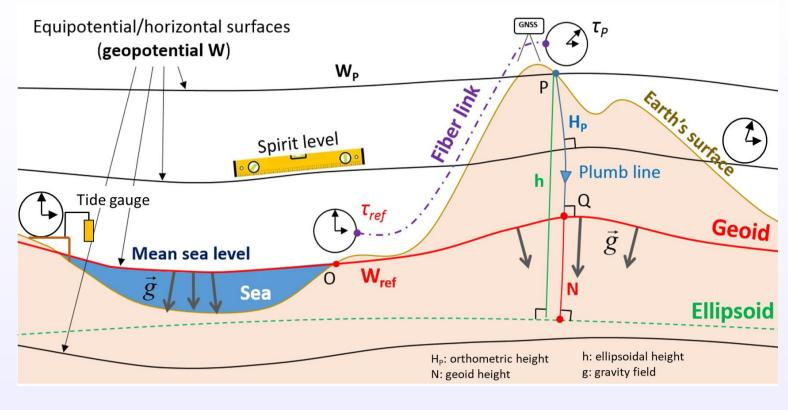
In turn, an atomic clock travelling in the field can be used to perform a cartography of the geopotential,
