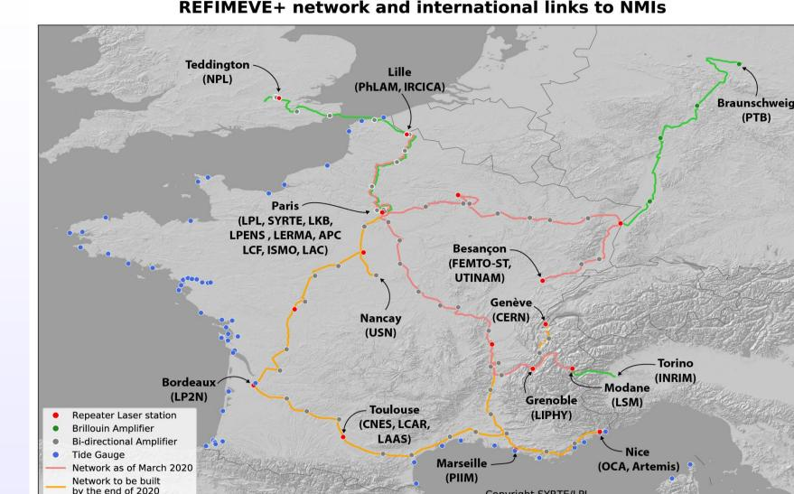
The Equipex **REFIMEVE+** disseminates a **1542 nm ultrastable IR carrier** throughout France, with connections to corresponding networks in Germany, UK and Italy. Phase noise due to propagation is
