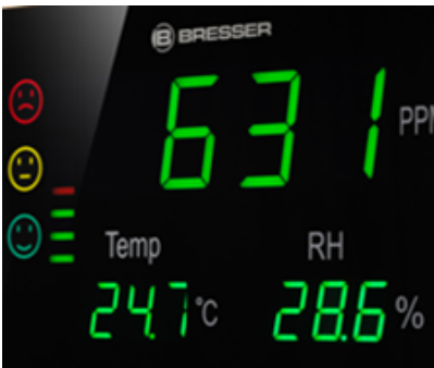
New devices to measure CO2, Humidity and Temperature at the reading room
