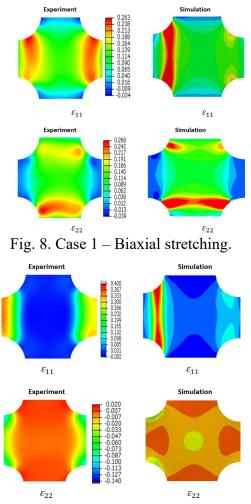
*Fig. 9. Case 2 – Near plane strain condition.*
