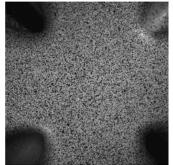
Fig. 5. Random speckle pattern applied on the top surface of the gauge region.
