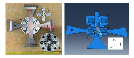
*Fig. 6. Components of punching die and view of the 3D model assembly:* A - base part; B - cross holder; C - upper part; D - 0.5 mm cruciform sample.
