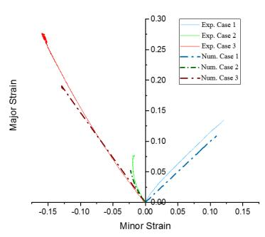
Fig. 11. Comparison of the strain paths for the three loading conditions.
