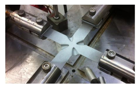
Fig. 4. Experimental setup with the pre-deformed cruciform sample.
