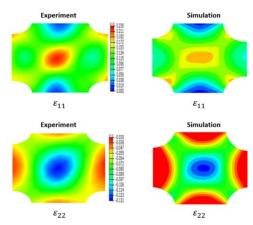
Fig 10. Case 3 – Uniaxial stretching.
