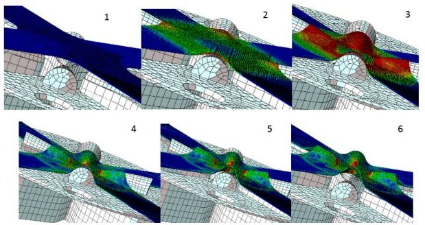
Fig. 2. Cruciform sample preforming (1 to 6 - successive steps).
