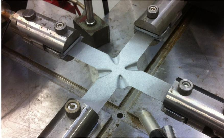
*Fig. 4. Experimental setup with the pre-deformed cruciform sample.*
