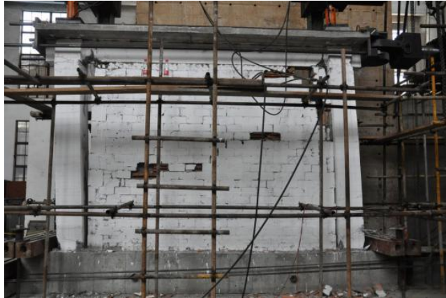
Figure 6 Damage of Specimen 3 at R = 4%
