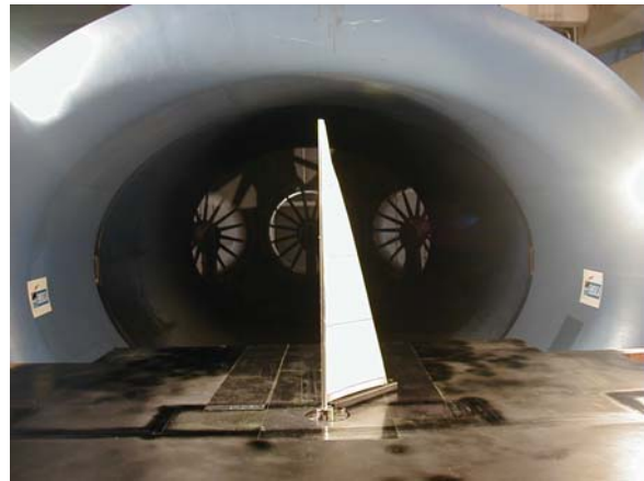
Figure 21: S4 wind-tunnel test section in aerodynamic sail force measurements configuration.
