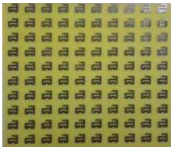
Fig.2.Fabricated FSS with an array of 10 \times 10 unit cells.
