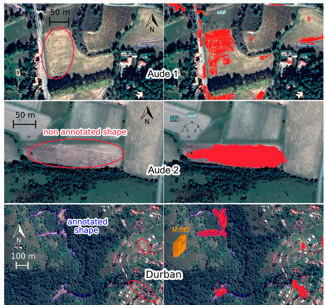
Figure 11. Illustrations of missing annotated shapes (red ovals in the left images) that were correctly detected using the FuSVIPR method (either U-net or RF in the right images) in Aude 1, Aude 2 and Durban. Such configurations induced spurious rises in the FPRs. Hence, all FPRs given in this study systematically constituted upper limit values. In this figure, blue lines and red pixels depict the ground truths and PFs detected through FuSVIPR, respectively.
