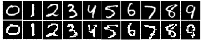
Fig. 8: First line: original MNIST images fed to the BNN. Second line: recovered images from Bus ECG with 200 averaged traces
