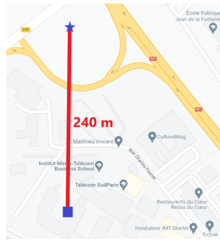
Figure 10. The true position corresponding to the “real” signals and the “fake” one corresponding to the spoofer signal.
