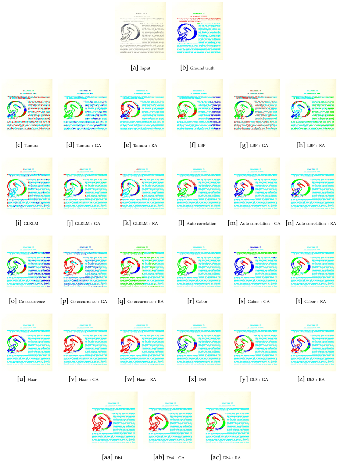
Figure 7. Resulting pixel-labeling images without and with using a feature selection algorithm on a historical document image of the “Three fonts and graphics” category from the testing dataset of the HBR2013 dataset . The number of class labels is equal to 4. Since the pixel-labeling task is unsupervised, the colors attributed to text or graphics may differ from one document to another. Figures 7[a] and 7[b] illustrate the input image and its associated ground truth, respectively. The remaining figures depict the resulting pixel-labeling images.
