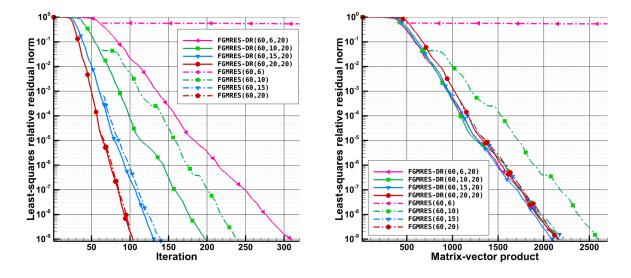
Figure 8: Impact of deflation for various sizes of the inner Krylov space for FV case. Adjoint relative residual norm convergence history with respect to iterations (left) and Jacobian-vector products (right) for FGMRES(60, mi) and FGMRES-DR(60, mi, 20) with mi = 6, 10, 15, 20.
