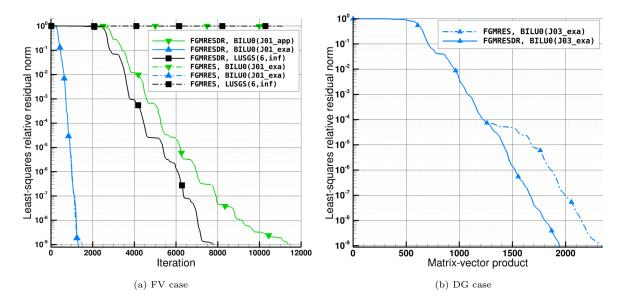
Figure 2: Impact of deflation for various preconditioners. The relative residual norm convergence history is plotted with respect to iterations. The impact of deflation is dramatically effective both on the LUSGS and BILU preconditioners applied to the first-order approximate Jacobian matrix. We recall the numerical parameters of the FGMRES-DR solver as follows:  $m = 60, m_i = 20$  and k = 20.
