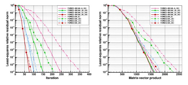
Figure 9: Impact of deflation for various sizes of the inner Krylov space for DG case. Adjoint relative residual norm convergence history with respect to iterations (left) and Jacobian-vector products (right) for FGMRES(60, mi) and FGMRES-DR(60, mi, 20) with mi = 6, 10, 15, 20.
