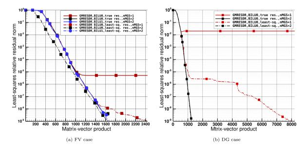
Figure 5: True and least-squares residual norm convergence histories by applying two steps of Gram-Schmidt orthogonalization procedure: *least-sq. res.* stands for least-squares residual while *true res.* stands for true residual. We recall the numerical parameters of the GMRES-DR solver as follows: m = 140 and k = 42
