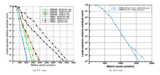
Figure 7: Impact of deflation for various preconditioners. The relative residual norm convergence history is plotted with respect to Jacobian-vector products. The hierarchy of the preconditioners remains the same as the one in Figure 6.
