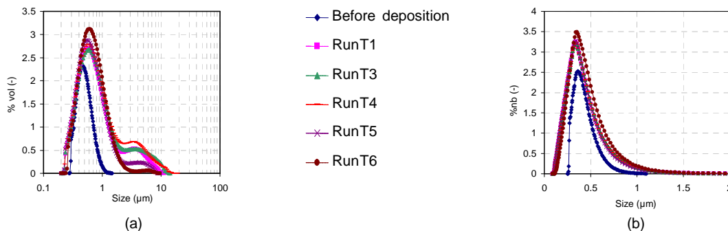
Figure 2: Size distribution of uncoated and Si-coated TiO 2 powders measured by laser granulometer. a) volumetric percentages, b) total number of particles percentages.
