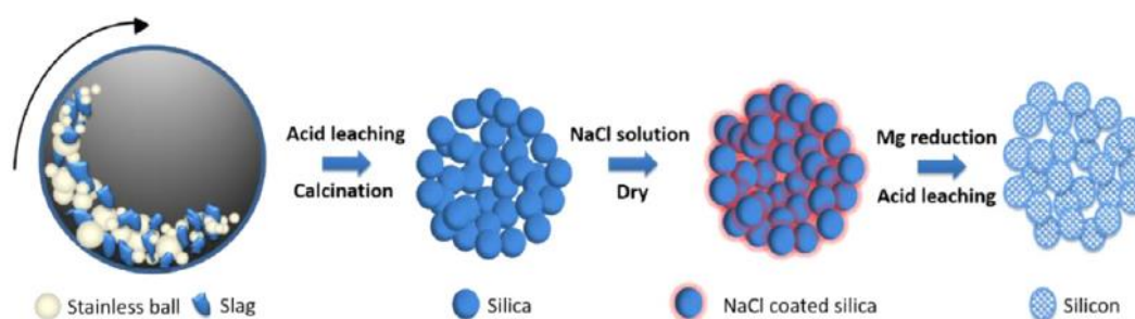
Fig. 46. Scheme of the method to prepare porous silicon from sodium slag (Huang et al. 2018).
