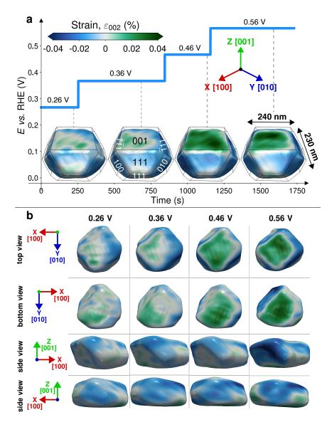
Figure 2. Revealing the influence of the electrode potential on the surface strain ( $\varepsilon_{002}$ ). Panels **a** and **b** present the same particle viewed from different perspectives. The colour bar is identical across the panels **a** and **b**. See Supplementary Figure 4 for multiple views of the reconstructed phase at different electrode potentials.
