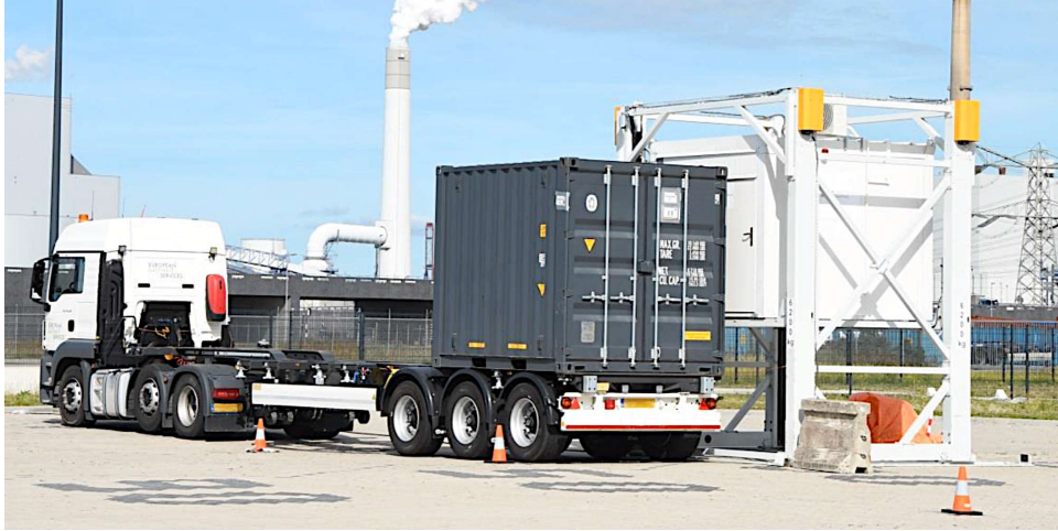
Slika 3: RRTNIS inspecting a standard 10 ft cargo container during the Rotterdam field trials.
