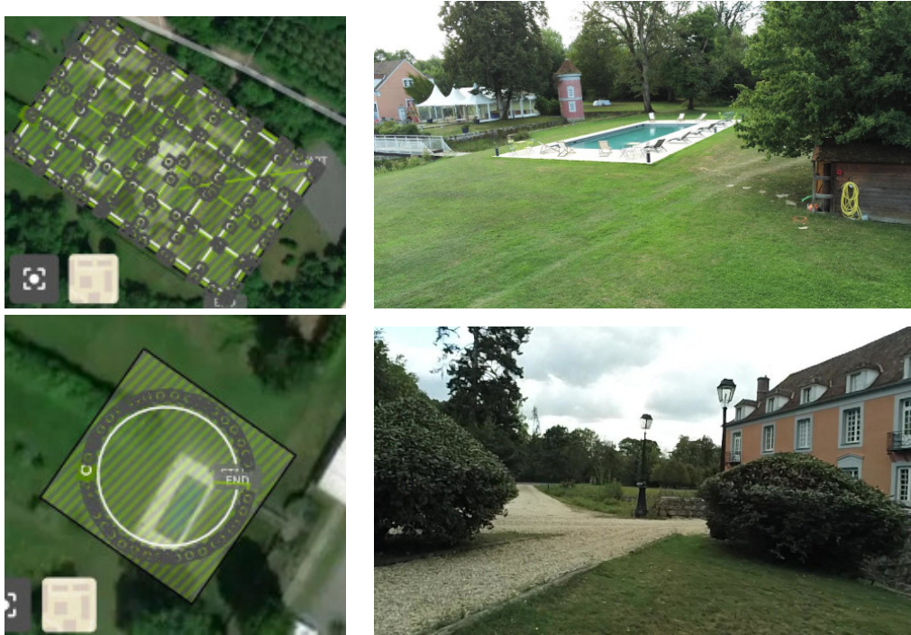
Fig. 7 Video acquisition process of the Manoir dataset. Left: grid (top) and orbit (bottom) flight plan used for photogrammetry. Right: Video samples from the Anafi drone, 4k (top) and 720p (bottom).
