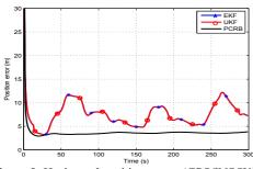
Figure 5: Horizontal position errors (GPS/INS/WSS).
