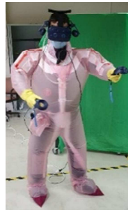
Figure 6 – Air Fed Suit Mixed Reality prototype for simulation
