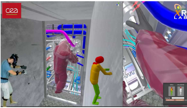
Figure 10 – Bolts Accessibility Study with eXtended Reality
