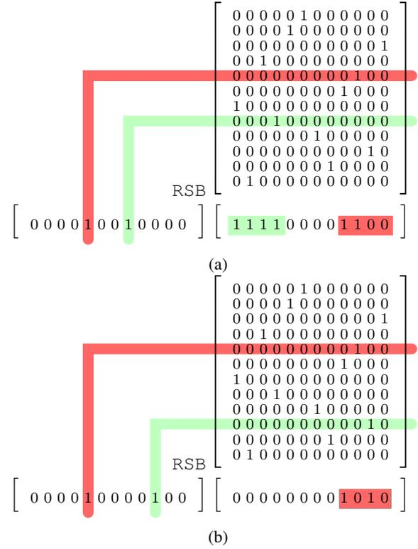
Figure 4: Illustration of faulty multiplications between a vector and a permutation matrix, with EOR replaced by RSB. Figure 4a triggers an error or corruption, whereas Figure 4b does not.
