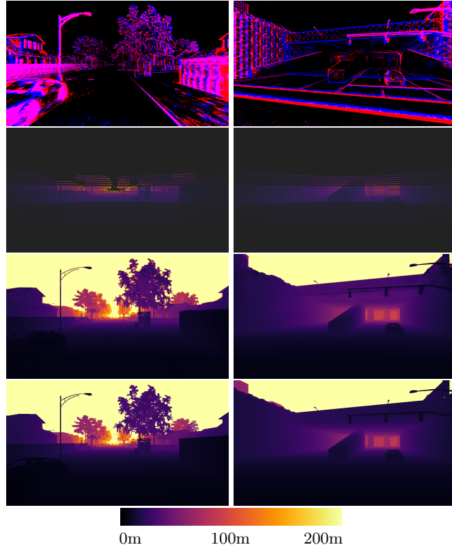
Fig. 4: Two qualitative results on our synthetic SLED dataset, on Town01 (left) and Town02 (right). From top to bottom: events, LiDAR, predicted depth map, ground truth, color scale.
