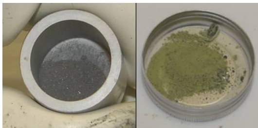
Fig. 8: Pictures of the powder before chlorination and after second chlorination at 150°C.
