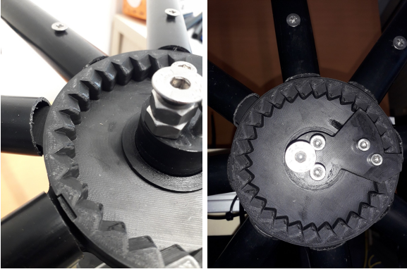
Figure 5: Freewheel with angled teeth.
