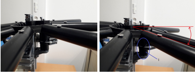
Figure 6: Left: lock gripper. Right: unlock gripper when the torque becomes too high. 1: spring (inside a guide tube) to maintain the rotating part at the horizontal in contact with the pawl when the gripper is locked.
