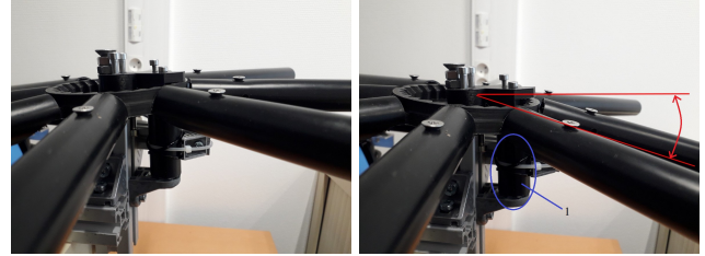
Figure 6: Left: lock gripper. Right: unlock gripper when the torque becomes too high. 1: spring (inside a guide tube) to maintain the rotating part at the horizontal in contact with the pawl when the gripper is lock.
