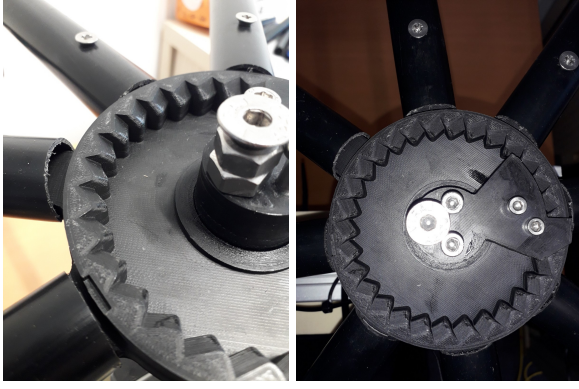
Figure 5: Freewheel with angled teeth.
