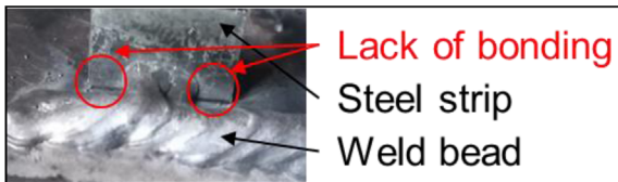
Fig. 4. Steel strip not well bonded with the deposited bead for offset > 3.0 mm.
