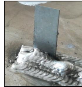
Fig. 18. Steel strip completely inserted between several layers.
