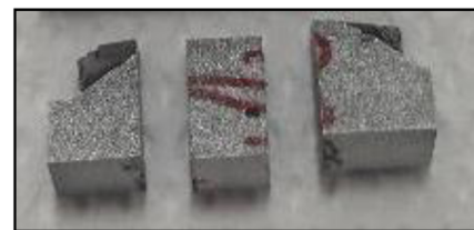
Fig. 14. Middle of the sample realized with a 2.5 mm offset isolated for SEM inspection.
