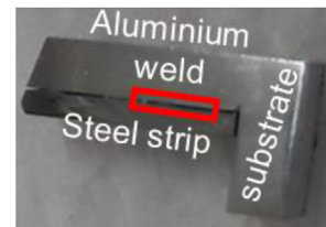
Fig. 15. Samples prepared for SEM inspection with the area inspected identified in red.
