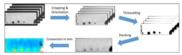
Fig. 7. Strip thickness map creation process.
