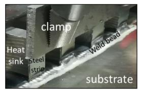
Fig. 2. Pictures of the experimental setup.
