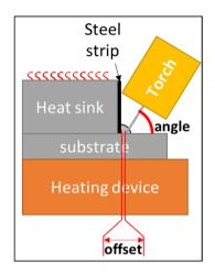
Fig. 1. Experimental set up.
