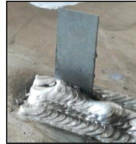
**Fig. 18.** Steel strip completely inserted between several layers.
