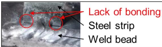
**Fig. 4.** Steel strip not well bonded with the deposited bead for offset > 3.0 mm.
