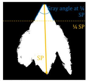
**Figure 2.** Definition of spray characteristics for the liquid spray of ethanol as an example
