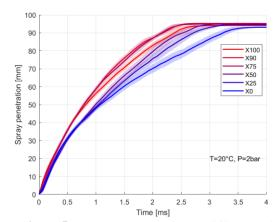
**Figure 5.** Spray penetration for the different ratio of ammonia
