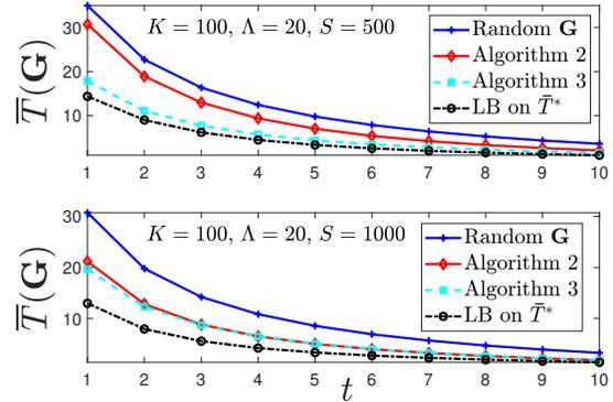
Fig. 7:  $\bar{T}(\mathbf{G})$  of random user-to-cache state association, the user-to-cache state associations obtained from **Algorithm 2**, and **Algorithm 3** from (17), and the lower bound (LB) of (18).
