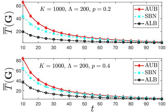
Fig. 3: Analytical upper bound (AUB) from (13) vs. analytical lower bound (ALB) from (14) vs. sampling-based numerical (SBN) approximation in (20) (for  $|\mathcal{L}_1| = 20000$  and uniform user-to-cache state association).
