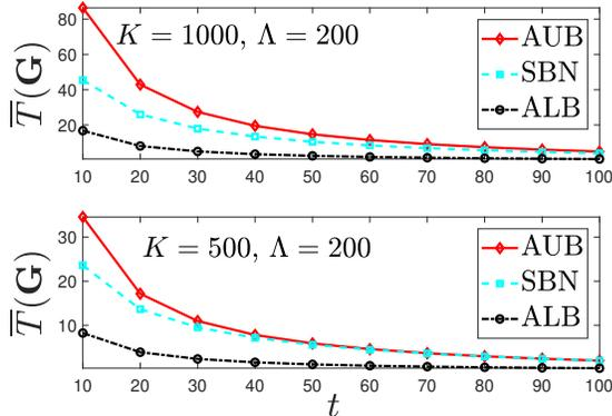
Fig. 2: Analytical upper bound (AUB) from (6) vs. analytical lower bound (ALB) from (7) vs. sampling-based numerical (SBN) approximation in (20) (for  $|\mathcal{L}_1| = 20000$ ,  $\mathbf{p}$  in (21), and random user-to-cache state association).
