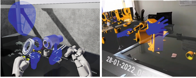
Fig. 7. MR collaboration between two users on an assembly task [67]. Right: VR environment with virtual hands replacing the controllers. Left: AR environment including hand tracking and virtual assembly parts which will be mapped to the physical parts. Source: own representation from Asynchronous manual work in mixed reality remote collaboration , Mayer et al. 2022.
