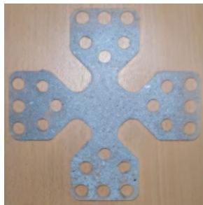
Fig. 3. Cruciform silicone specimen
