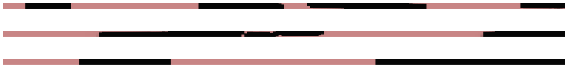
Fig. 12. Optimal solutions of the visco-elastic layer of the 2D sandwich beam (black: x_e > 0.99 ) for the displacement criteria, from bottom to top: \tilde{\underline{x}}_{500 \text{ Hz}}^d , \tilde{\underline{x}}_{1000 \text{ Hz}}^d , \tilde{\underline{x}}_{2000 \text{ Hz}}^d .
