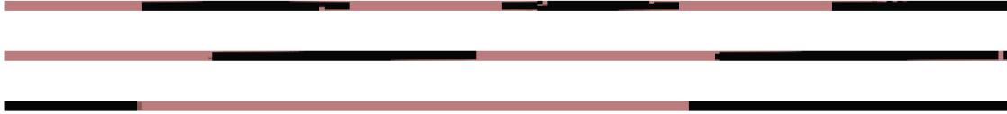
Fig. 9. Optimal solutions of the visco-elastic layer of the 2D sandwich beam (black: x_e > 0.99 ) for the compliance criteria, from bottom to top: \tilde{x}_{500 \text{ Hz}}^c , \tilde{x}_{1000 \text{ Hz}}^c , \tilde{x}_{2000 \text{ Hz}}^c .
