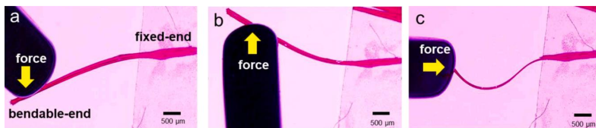
Fig. 6. Mechanically flexible characteristics of long crystal of 1 . Crystal size: 5.13 cm (length) \times 200 \mu\text{m} (width) \times 50 \mu\text{m} (thickness).
