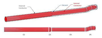
Fig. 5. Top – The design of the impedance transformer, where in red the inner conductor is represented, in blue the vacuum volume, and in dashed black the outer conductor. Bottom – The cut view representation of each of the impedance transformer multipactor regions. The impedance transformer is divided into four different multipactor regions: (1) – Section 1, (2) – Transition 1, (3) – Section 2, and (4) – Transition 2.
