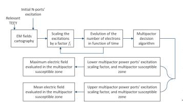
Fig. 7. The steps summarizing the applied methodology for the determination of the multipactor electric fields thresholds for each of the components' regions.
