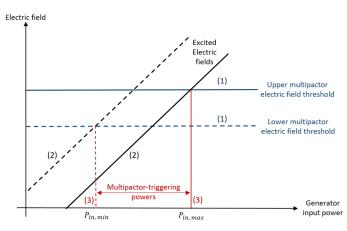
Fig. 3. Illustration of the main three steps used to solve the problem for a given frequency. The blue lines correspond to the electric field multipactor thresholds, the black lines correspond to the excited electric fields, and the red lines correspond to the resultant generators' forward powers triggering multipactor inside the geometry.
