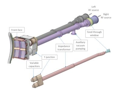
Fig. 1. Top – An illustration of the different components of one ICRH antenna used on the tokamak WEST. Each side has its own high-power generator. Bottom – The inner conductor representation of the feed-through window, impedance transformer, and T-junction.
