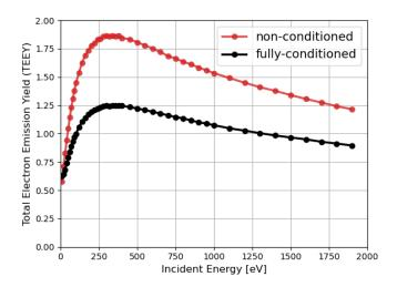
Fig. 2. TEEY measurements for a baked WEST ICRH representative silver-coated sample, maintained at  $70\,^{\circ}$ C. In red, the TEEY data are measured before any conditioning treatment; and in black, the TEEY data are measured after a full conditioning treatment of the surface (with a cumulative electron dose of  $2338\,\mu\mathrm{C}\,\mathrm{mm}^{-2}$ ) [19].
