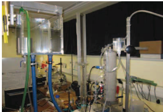
Two views of sand column with tensiometers, TDR probe, and (below) the reservoir.
