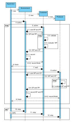
Figure 2. Sequence diagram of SCEP model
