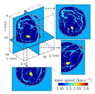
**Fig. 2.** Three-dimensional wave speed model of size  $10 \times 16 \times 16 \text{cm}^3$  that corresponds to binary file 3D/models/main/cp\_121  $\times$  191  $\times$  201.bin. We picture the cross-sections corresponding to y-z plane (top right), x-z plane (bottom right) and x-y plane (bottom left). In the numerical simulations with wall conditions, an absorbing boundary condition is imposed on the y-z plane for  $x=x_{max}=10 \text{cm}$ , to mimic the body.
