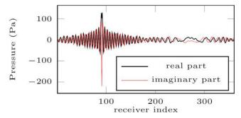
**Fig. 3.** Pressure field saved for the 2D case at frequency 200kHz for the source numbered 10, in the configuration of absorbing boundary conditions with Kelvin–Voigt model of attenuation. It corresponds to file 2D/wave-dataset /data\_absorbing-boundary-conditions/kelvin-voigt/receivers/data-record\_p\_frequency\_0.00000E+00\_2.00000E+05Hz\_src 000010.txt.
