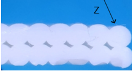
Fig. 11: Slice of a silicone print with \phi = 10^\circ with the nozzle axis: z axis of the nozzle
