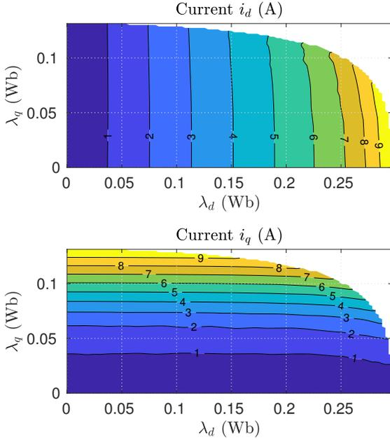
Fig. 6. Nonlinear current-flux characteristic obtained from numerical inversion.
