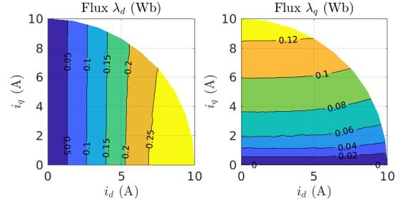
Fig. 3. Nonlinear flux-current characteristic obtained from FEMM.
