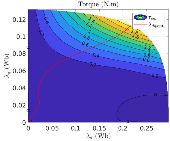
Fig. 7. Torque-flux characteristic and MTPA trajectory (red).
