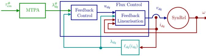
Fig. 10. Representation of the overall control scheme.
