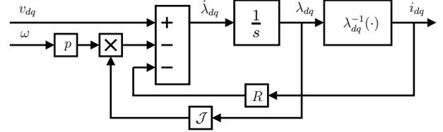
Fig. 5. Simulation model of the flux dynamics (2).
