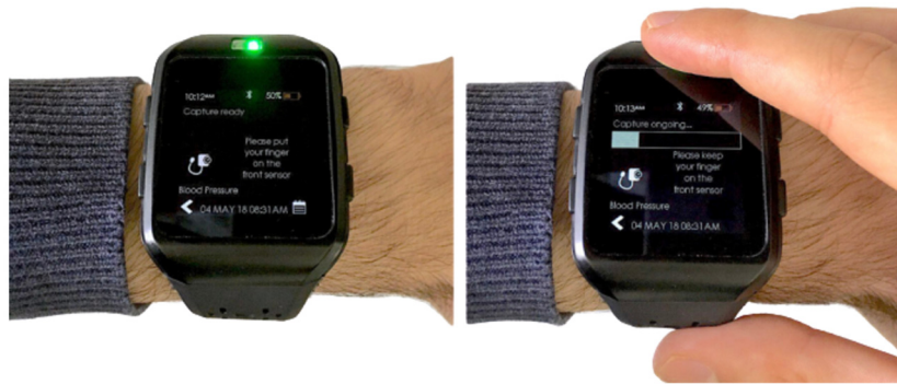
Fig. 3. CareUp performing blood pressure estimation.
