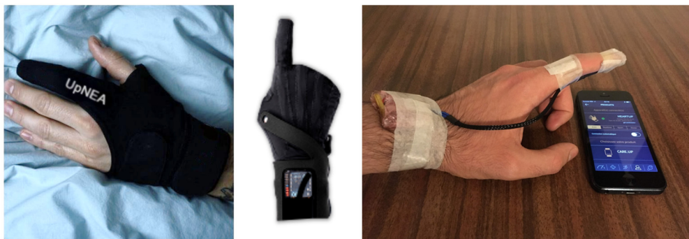
Fig. 4. The UpNEA device and its prototype.
