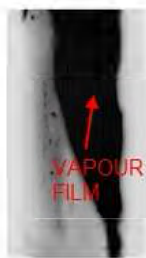
FIGURE 10. FILM BOILING ON THE METAL FOIL, IR CAMERA IMAGE. THE VAPOUR FILM APPEARS FROM THE RIGHT CORNER.
