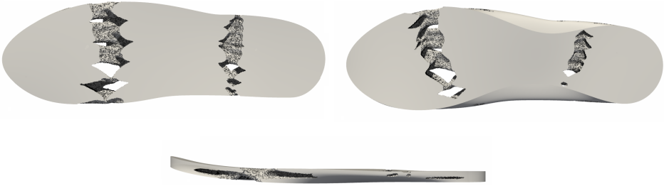
Fig. 20 Various views of the optimized sports shoe sole for the damping maximization of the structure.
