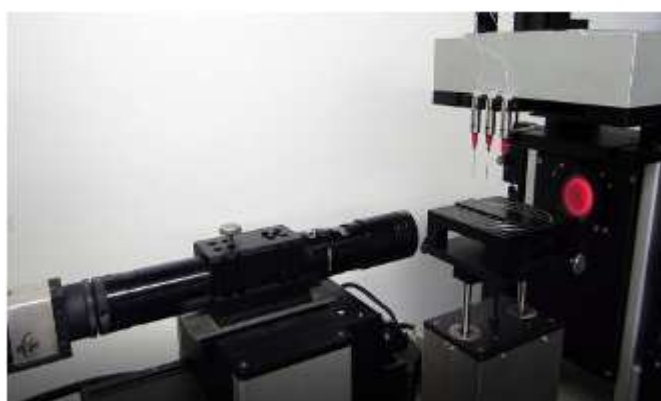
Figure 1: System of surface energy measurement
