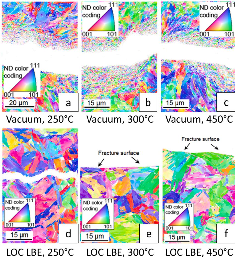
**Fig. 4.18.** EBSD<sup>†</sup> grain orientation maps in T91 F/M steels tested in vacuum at 250 °C, 300 °C, and 450 °C showing grain refinement along the crack wake, as opposed to testing in low-oxygen (LOC) liquid LBE at the same temperatures. Adapted from [500].
