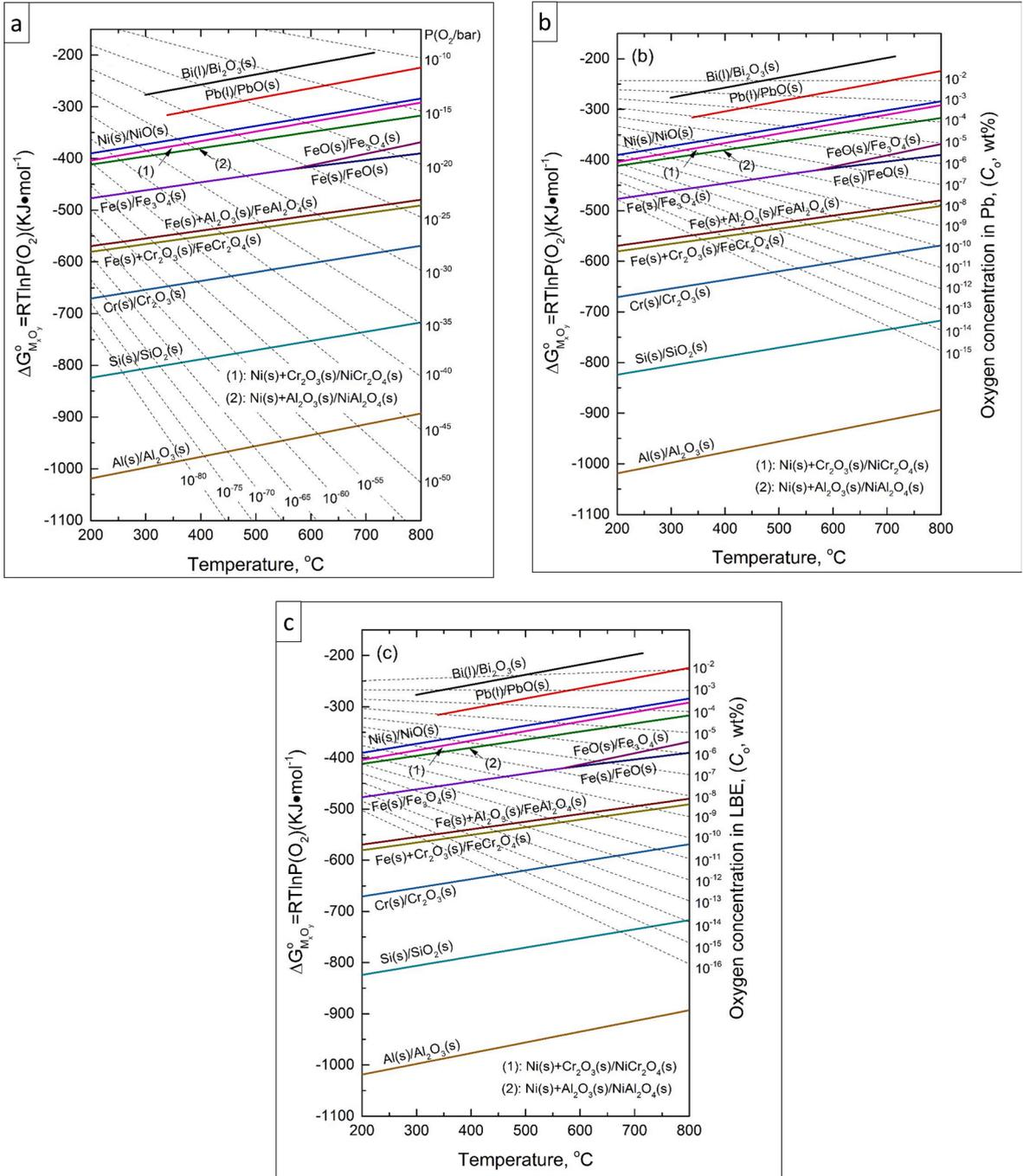
Fig. 3.9. Ellingham diagrams of the standard Gibbs free energy of oxide formation per mol O<sub>2</sub> (left y-axis) as a function of: (a) the oxygen partial pressure in the gas plenum above the HLM melt, (b,c) the concentration of dissolved oxygen in liquid Pb and liquid LBE, respectively, (right y-axis), and temperature (x-axis) for the formation of oxides due to the oxidation of the main steel alloying elements in liquid Pb and LBE. Adapted from [109].
