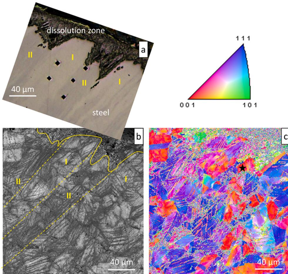
**Fig. 3.47.** (a) LOM<sup>†</sup> image of 60% CW 316L AuSS exposed to oxygen-poor ( $C_O < 10^{-11}$  wt%), static LBE at  $500\ ^\circ\text{C}$  for 1000 h: I – bands with higher Ni content, II – bands with lower Ni content. (b-c) EBSD<sup>†</sup> analysis shows that the segregation of defects is higher in the bands with lower Ni content. Adapted from [42].
