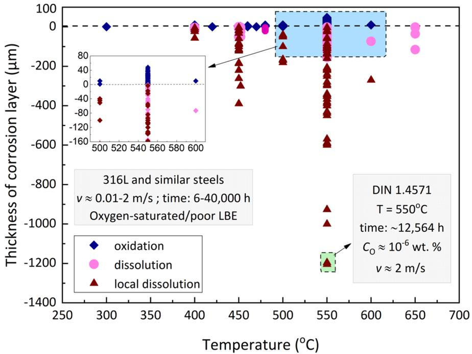
**Fig. 3.27.** Corrosion layer thickness in 316L AuSS and similar steels (304L, 316Ti, 15-15Ti) exposed to *flowing* HLMs as a function of the exposure temperature. The magnified inset shows data acquired in the 500–600 °C range and corresponding to corrosion layer thicknesses between –160 μm and 80 μm. Data collected from Refs. [43,44,95,96,102,104,106,115,118,141,172,180,187–189,191,214–230].
