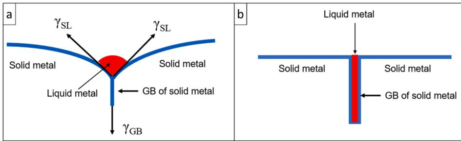
Fig. 4.1. GBW<sup>1</sup> at the interface between a liquid metal and a solid metal: (a)  $2\gamma_{SL} > \gamma_{GB}$ ; (b)  $2\gamma_{SL} < \gamma_{GB}$ .
