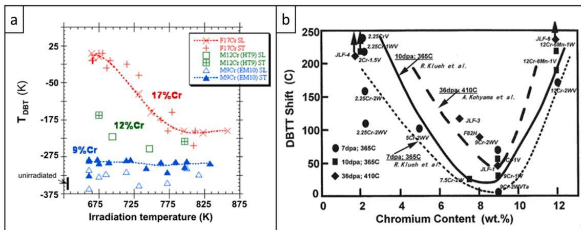
Fig. 2.1. (a)  $DBTT^{\dagger}$  of 9Cr, 12Cr, and 17Cr F/M steels after neutron irradiation at different temperatures [46]. (b)  $DBTT$  shift of low-activation ferritic steels, as a function of the steel Cr content, after neutron irradiation in the FFTF†. Adapted from [50].
