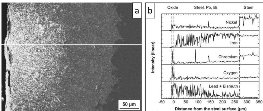
Fig. 3.19. (a) SEM<sup>†</sup> image of the dissolution-affected zone in 316L AuSS exposed to flowing LBE ( $v \approx 2$  m/s,  $C_0 \approx 1.6 \times 10^{-6}$  wt%) at 550 °C for 7518 h. (b) The EDS<sup>†</sup> line scan along the white line in (a) reveals the selective leaching of Ni and Cr. Adapted from [115].
