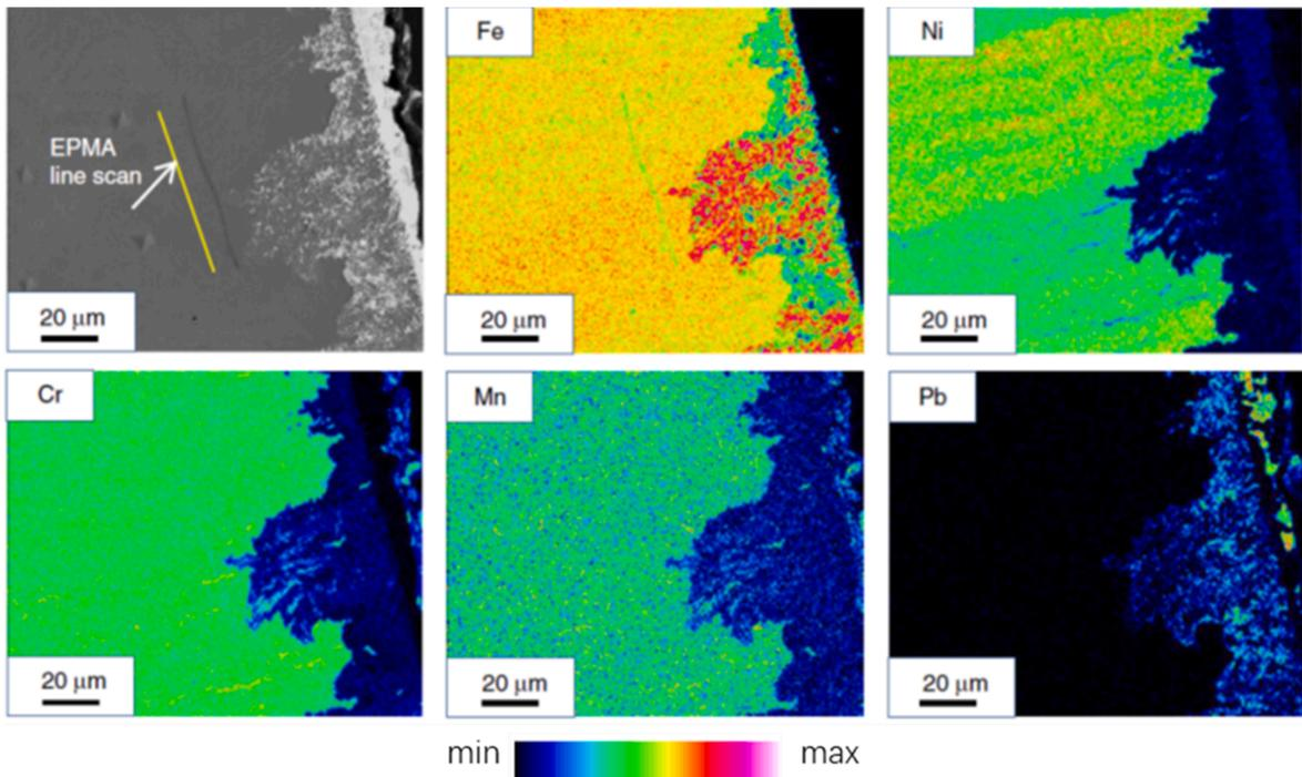
Fig. 3.43. EPMA<sup>†</sup> elemental maps showing the correlation of chemical bands with the local LBE dissolution attack in a SA 316L AuSS exposed to oxygen-poor ( $C_O < 10^{-11}$  wt%), static LBE at 500 °C for 1000 h. Bands poorer in Ni are more attacked than bands richer in Ni. Adapted from [177].
