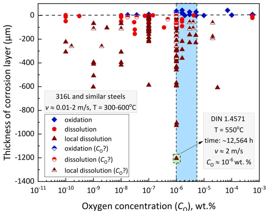
Fig. 3.37. Corrosion layer thickness in 316L AuSS and similar steels (316, 1.4571, 18Cr-10Ni-Ti, 08  $\times$  16H11M3) as a function of the oxygen content in *flowing* HLMs. Data corresponding to uncertain HLM oxygen contents are indicated by special symbols and “ $C_O?$ ” in the figure legend. Data collected from Refs. [43,44,95,96,102,104,106,115,118,141,172,180,187–189,191,214–230].
