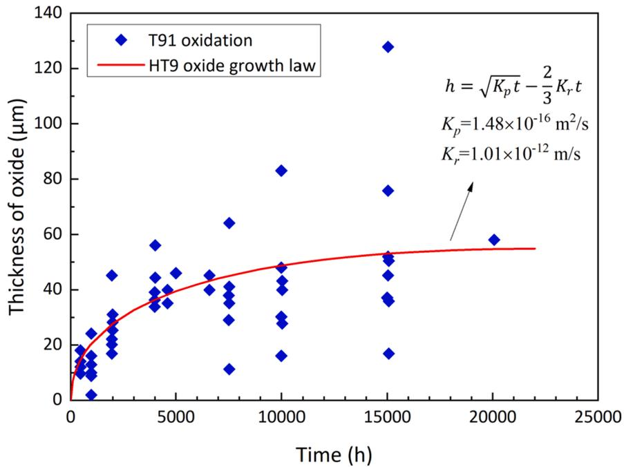
**Fig. 3.35.** Thickness of oxide scales on T91 F/M steels as a function of exposure duration in *flowing* LBE. All data resulted from steel exposures at  $550^\circ\text{C}$  to oxygen-containing LBE ( $C_{\text{O}} \approx 10^{-6}\text{--}10^{-5}$  wt%). The red curve corresponds to the oxide scale growth law suggested for HT-9 F/M steels by Zhang [30,134]. (For interpretation of the references to colour in this figure legend, the reader is referred to the web version of this article.)
