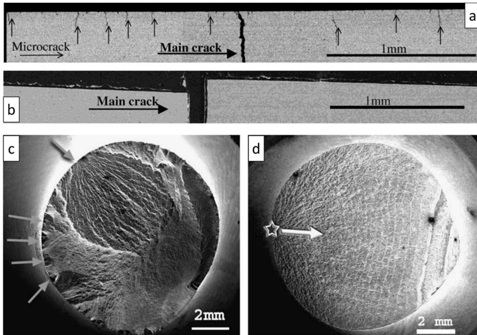
**Fig. 4.34.** SEM<sup>†</sup> images showing (a) multiple cracks on the surface of a T91 F/M steel specimen tested in low-cycle fatigue in air, as opposed to a single crack on a specimen tested in liquid LBE at 300 °C (b). (c,d) Fractography shows multiple crack initiation sites for the specimen tested in air, but a single crack initiation site for the specimen tested in liquid LBE. Adapted from [509,529].
