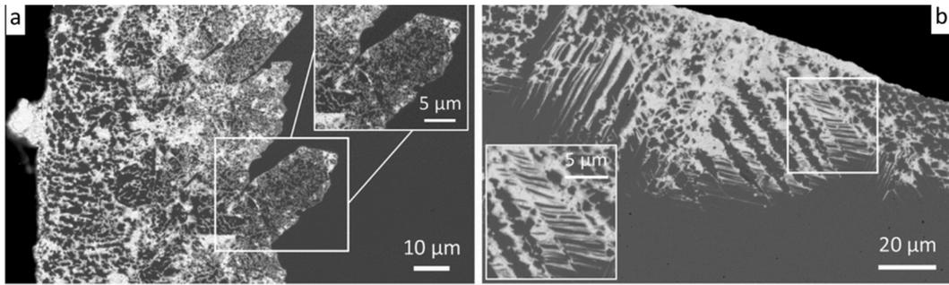
**Fig. 3.2.** SEM<sup>I</sup> images of 316L AuSS exposed to oxygen-poor ( $C_O < 10^{-8}$  wt%), static LBE at 500 °C: (a) a SA<sup>I</sup> steel exposed for 3282 h, and (b) a CW<sup>I</sup> steel exposed for 1000 h. The LBE does not penetrate into the 316L AuSS perpendicularly to the steel surface, but follows preferred ingress paths, such as grain/twin boundaries. Adapted from [40].
