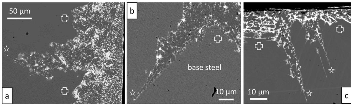
**Fig. 3.50.** SEM<sup>†</sup> images of sharp protrusions of the dissolution front in CW 316L AuSS exposed to oxygen-poor ( $C_O < 10^{-8}$  wt%) static LBE at 500 °C for (a) 3282 h, (b) 2055 h, and (c) 501 h. Adapted from [40].
