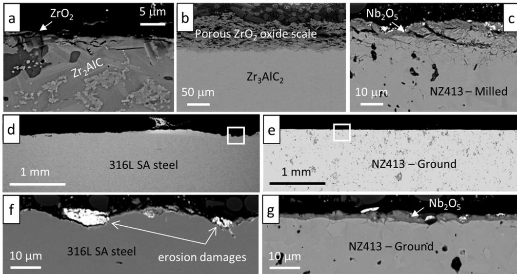
**Fig. 5.12.** SEM<sup>†</sup> images of materials exposed to fast-flowing ( $v \approx 8$  m/s), oxygen-poor ( $C_O \approx 5 \times 10^{-9}$  wt%) liquid LBE at 500 °C for 1000 h: (a)  $Zr_2AlC$ , (b)  $Zr_3AlC_2$ , (c)  $(Nb,Zr)_4AlC_3$  with milled surface finish, (d,f) SA 316L AuSS – overview & detail, (e,g)  $(Nb,Zr)_4AlC_3$  with ground surface finish – overview & detail. Adapted from [83].
