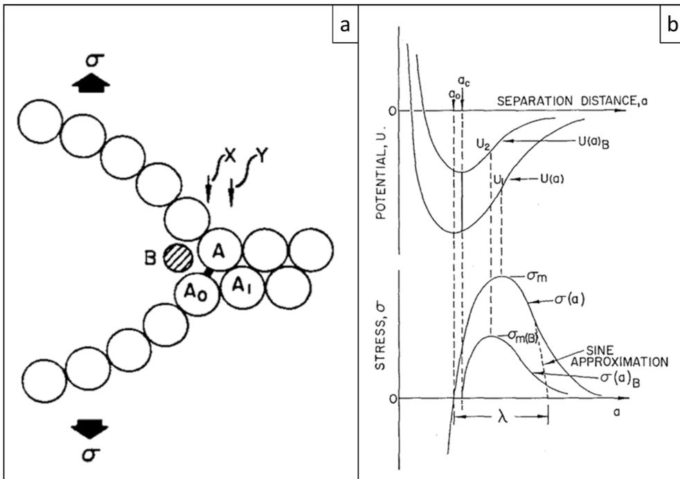
Fig. 4.8. Schematic illustration of the adsorption-induced reduction in cohesion model. (a) Atomic-scale process leading to the reduction of cohesion by breaking A-A<sub>0</sub> atomic bonds. (b) Schematic of the reduction in the magnitude of the interatomic potential and the associated, lowered stress required to overcome this potential energy barrier. Adapted from [362].
