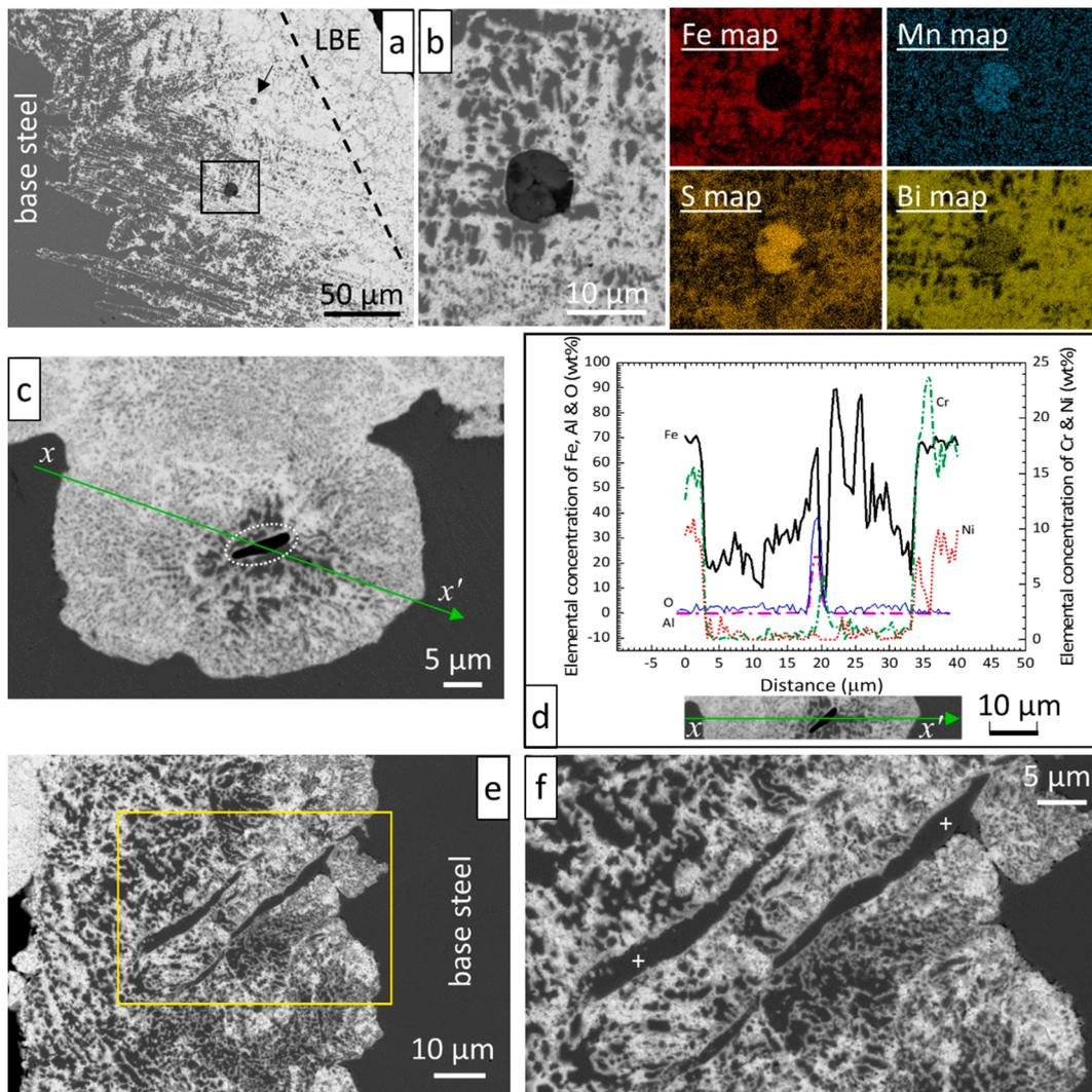
**Fig. 3.49.** SEM<sup>†</sup> images of precipitates in 316L AuSS exposed to oxygen-poor ( $C_O < 10^{-8}$  wt%), static liquid LBE at 500 °C for 3282 h: (a-b) MnS precipitates in CW 316L AuSS; (c-d) Al-rich oxide inclusion with corresponding EDS<sup>†</sup> line scan, and (e-f)  $\delta$ -ferrite stringers (crosses) in SA 316L AuSS. Adapted from [40].
