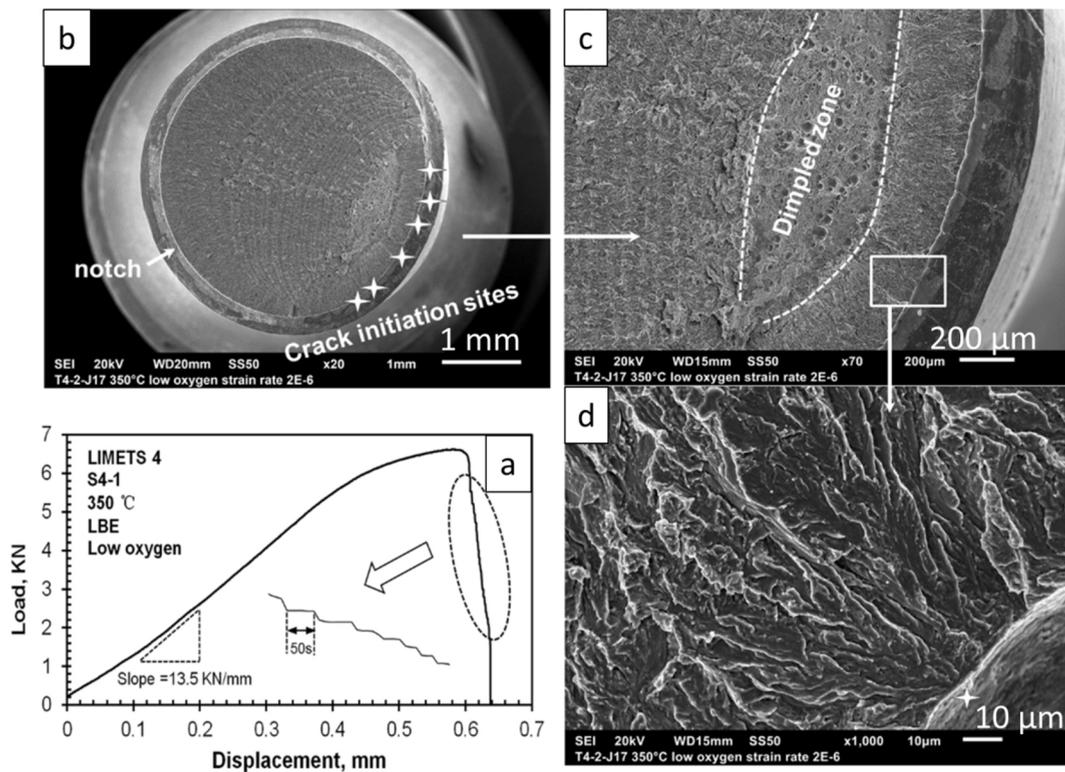
Fig. 4.41. SEM<sup>†</sup> images of T91 F/M steel fracture surfaces showing a mixture of LME-induced brittle fracture and ductile, dimple-rich fracture tested in low-oxygen liquid LBE at 350  $^{\circ}$ C. Adapted from [473].
