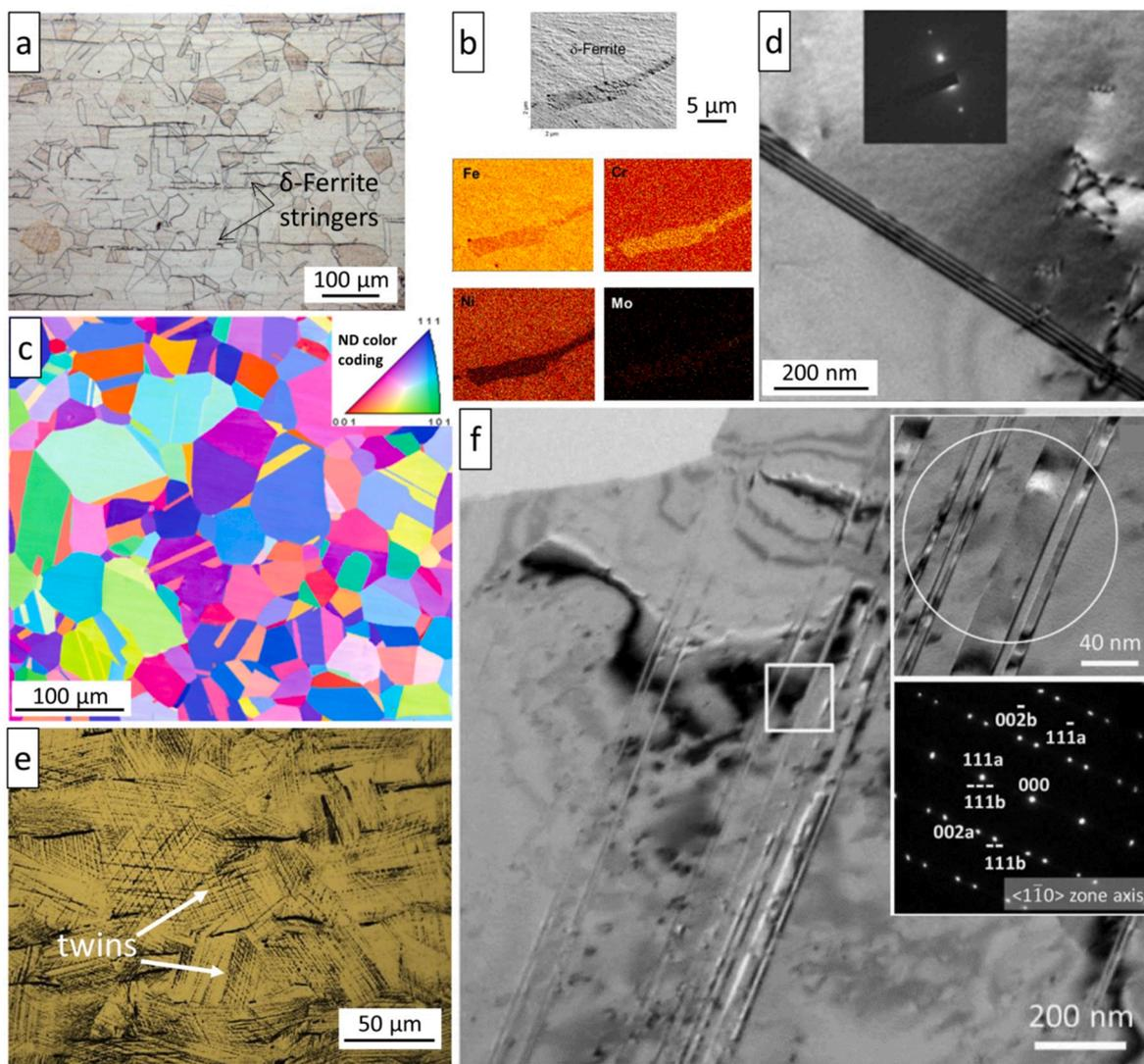
**Fig. 2.4.** Microstructure of SA<sup>†</sup> and CW<sup>†</sup> 316L AuSS. SA 316L: (a) LOM<sup>†</sup> image of  $\delta$ -ferrite stringers; (b) EDS<sup>†</sup> elemental maps of  $\delta$ -ferrite; (c) EBSD<sup>†</sup> grain orientation map; (d) TEM<sup>†</sup> BF image of nano-twins. CW 316L: (e) LOM image of deformation twins; (f) TEM BF images and SAED<sup>†</sup> pattern of deformation twins. Adapted from [40,58].
