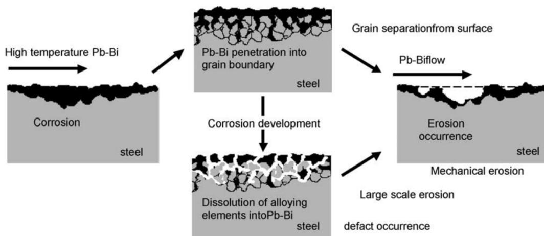
Fig. 3.25. Schematic illustration of an erosion/corrosion mechanism [191].
