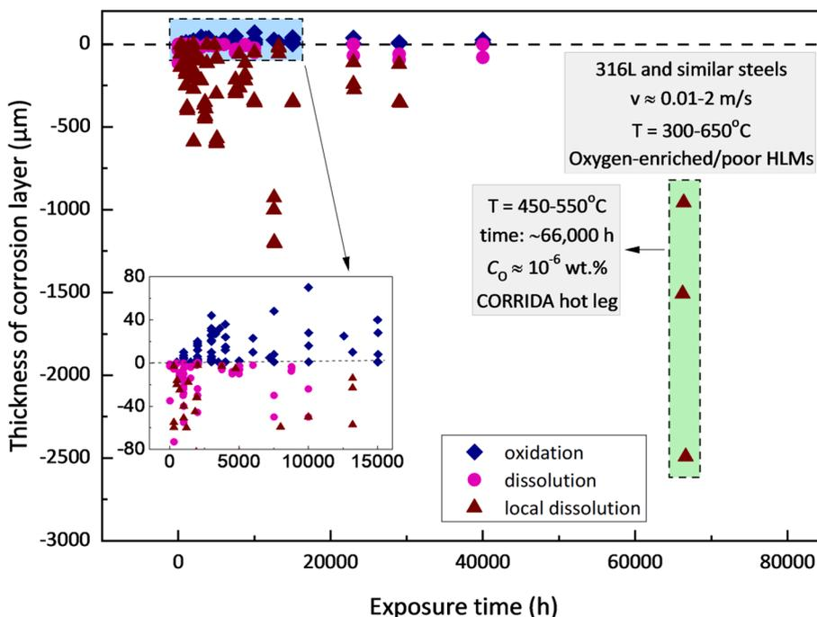
Fig. 3.32. Corrosion layer thickness in 316L AuSS and similar steels as a function of the duration of exposure to *flowing* HLMs. The magnified inset shows the evolution in corrosion layer thickness in the first 15,000 h of exposure and for corrosion layer thicknesses between  $-80$   $\mu\text{m}$  and  $80$   $\mu\text{m}$ . Data collected from Refs. [43,44,95,96,102,104,106,115,118,141,172,180,187–189,191,214–230].
