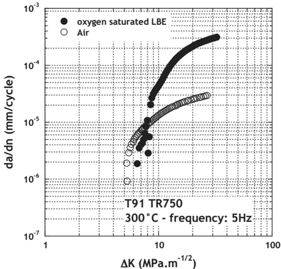
Fig. 4.38. Fatigue crack propagation rate ( $da/dn$ ) vs. stress intensity factor range ( $\Delta K$ ) for T91 F/M steels tested in oxygen-saturated liquid LBE and air at 300 °C; one cycle was 0.2 s [527].
