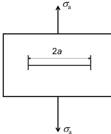
Fig. 4.7. Typical geometry used to describe the reduction in surface energy mechanism of LME, where a solid sheet containing a flat crack with a length of  $2a$  is remotely loaded by a stress  $\sigma_a$ .
