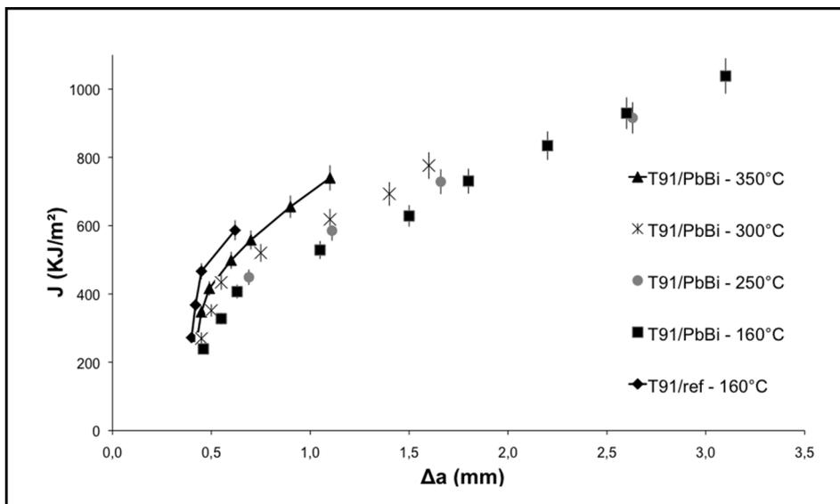
Fig. 4.22. J-R curves for T91 F/M steels exposed to liquid LBE under plane-stress loading conditions, using a CCT<sup>†</sup> specimen geometry [470].
