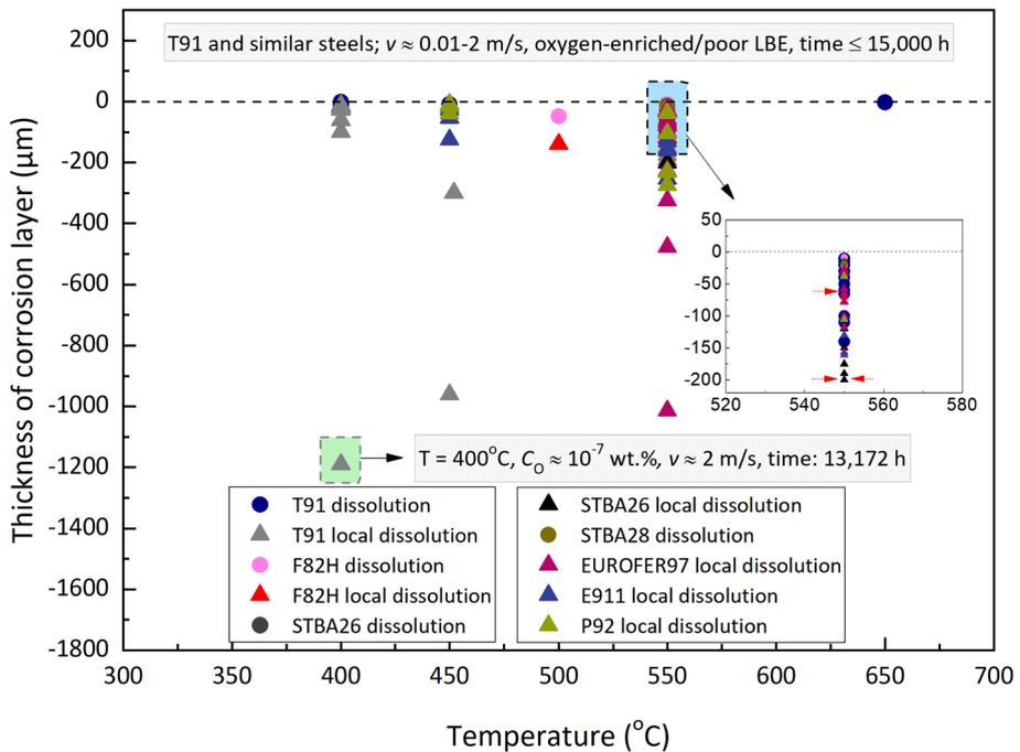
**Fig. 3.30.** Dissolution depths in T91 F/M and similar steels as a function of the exposure temperature in *flowing* LBE. The magnified inset shows data acquired at 550°C and corresponding to corrosion layer thicknesses between -200 μm and 50 μm. Data collected from Refs. [92,101,117,180,181,183,187,190,191,215–217,225,227,231,232]. Steel grades: T91, F82H, STBA26, STBA28, EUROFER-97, E911 and P92. Mechanisms: uniform dissolution (circles), and locally enhanced dissolution (triangles).
