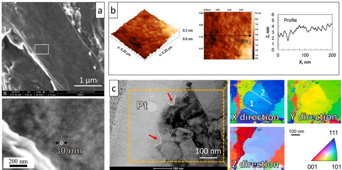
**Fig. 4.39.** (a) High-resolution SEM<sup>†</sup>, (b) AFM<sup>†</sup>, and (c) TEM<sup>†</sup> BF<sup>†</sup> images showing the presence of dimple-like structures on the micro/nanometre scales during trans-lath crack propagation in T91 F/M steels. Adapted from [53].
