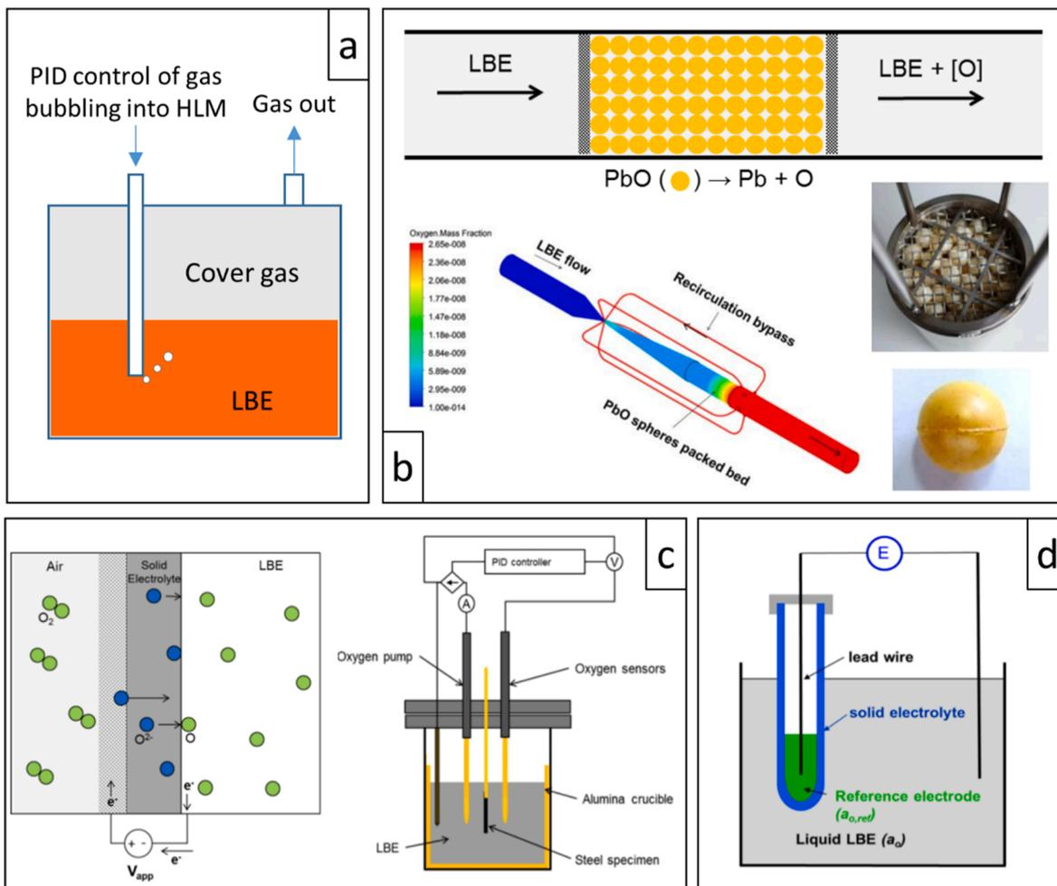
**Fig. 5.2.** (a) Schematic representation of automatic control by the supply of hydrogenated or oxygenated gases into the HLM bath. (b) A Venturi-type mass exchanger consisting of a packed bed of PbO solid spheres [577]. Working principles of (c) an electrochemical oxygen pump [575], and (d) an electrochemical oxygen sensor, adapted from [583].
