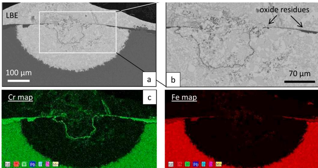
**Fig. 3.3.** (a-b) SEM<sup>I</sup> images of a deep (~227 μm) dissolution ‘pit’ in a EUROFER-97 F/M steel exposed to flowing ( $v \approx 1.8$  m/s) LBE with  $C_O \approx 2.3 \times 10^{-6}$  wt% at 550 °C for 3000 h. (c) EDS<sup>I</sup> elemental maps reveal residues of FeCr-spinel oxide scales still covering the largest part of this site of locally enhanced LBE dissolution attack. Adapted from [92].
