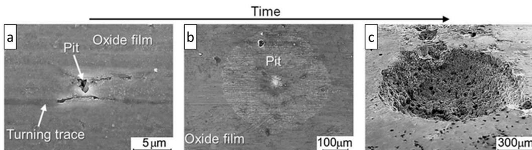
**Fig. 3.24.** SEM<sup>†</sup> images of the projected growth of ‘pits’ on the surface of 1.4970 and 1.4571 AuSS exposed to flowing LBE ( $v \approx 2$  m/s,  $C_O \approx 10^{-7}$  wt%). Adapted from [43].
