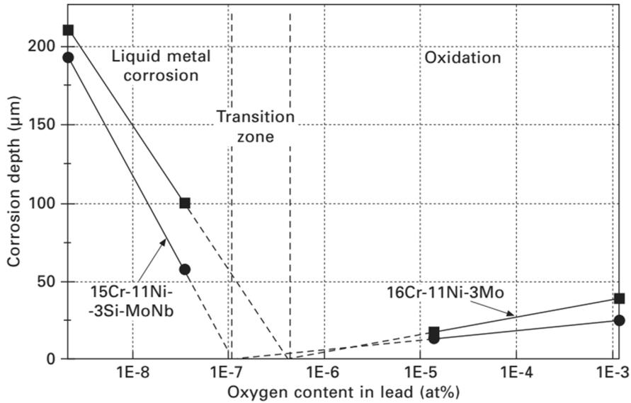
**Fig. 3.8.** Effect of the dissolved oxygen concentration on the LMC behaviour of two different AuSS exposed to liquid Pb for 3000 h at 550 °C [105,106]. Dissolution corrosion occurs at Pb oxygen concentrations  $<10^{-7}$  at%, while oxidation is the prevailing LMC mechanism at Pb oxygen concentrations  $>10^{-6}$  at%.
