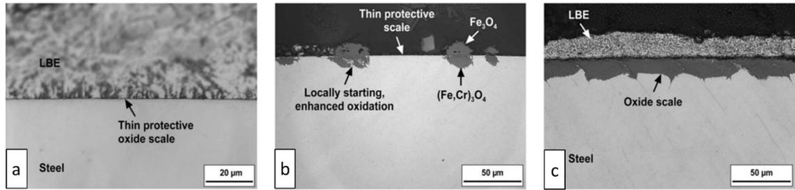
Fig. 3.14. SEM<sup>†</sup> images of oxide scale growth on 316L AuSS exposed to flowing LBE ( $v \approx 2$  m/s) with  $C_O \approx 1.6 \times 10^{-6}$  wt% at 550 °C for: (a) 503 h, (b) 4015 h, (c) 15,028 h. Adapted from [115].
