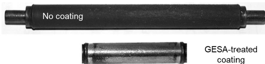
**Fig. 5.5.** Visual comparison of the surface appearance of T91 F/M steel fuel cladding tubes with and without GESA-treated FeCrAlY coatings after exposure to flowing ( $v \approx 1\text{--}1.2$  m/s) liquid LBE at  $550^\circ\text{C}$  for 2000 h. The surface of the fuel cladding tube without surface modification is dark, while the surface of the modified tube is shiny, showing the superior LMC resistance of the latter [192].
