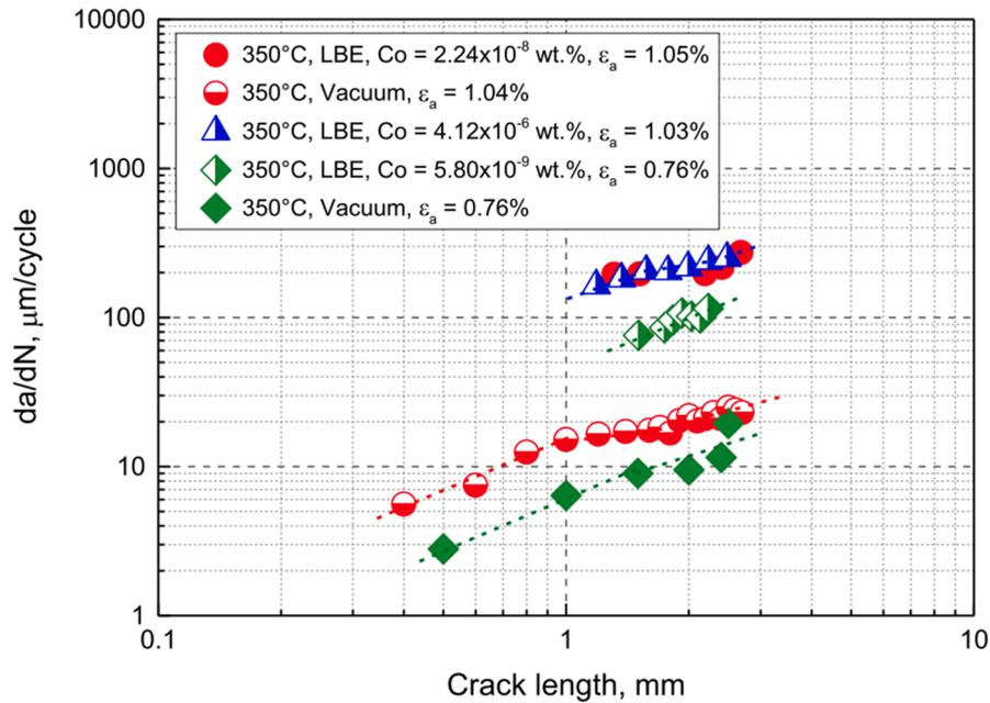
**Fig. 4.27.** Low-cycle fatigue crack propagation rates ( $da/dN$ ) for T91 F/M steels in vacuum, oxygen-rich ( $C_O \approx 4.12 \times 10^{-6}$  wt%) and oxygen-poor ( $C_O \approx 5.80 \times 10^{-9}$ – $2.24 \times 10^{-8}$  wt%) liquid LBE at 350 °C. The  $da/dN$  data were obtained from the fractographic examination of fatigue striations, where the space between two neighbouring striations corresponds to one cycle, assuming that there is no crack-closure effect [508].
