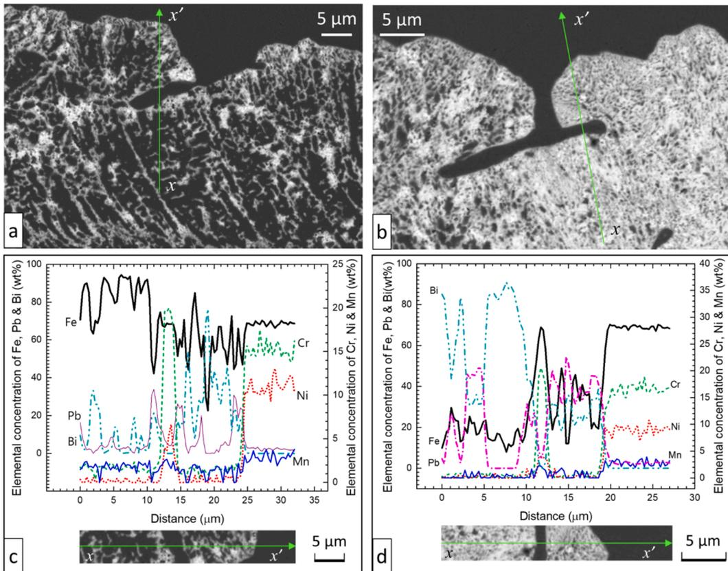
Fig. 3.44. SEM<sup>†</sup> images and EDS<sup>†</sup> line scans of the dissolution front in a SA 316L AuSS exposed to oxygen-poor ( $C_O < 10^{-8}$  wt%) static LBE at 500 °C for 3282 h: (a,c) selective leaching of Ni, Mn and Cr; (b,d) non-selective leaching of Ni, Mn, Cr and Fe. This steel specimen was fabricated from the same SA 316L AuSS heat showing chemical banding in Fig. 3.43. Adapted from [40].
