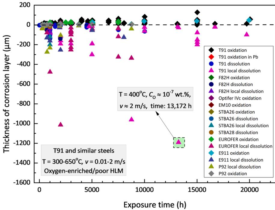
**Fig. 3.34.** Corrosion layer thickness in T91 F/M and similar steels as a function of the exposure duration in *flowing* HLMs. Steel grades: T91, F82H, Optifer IVc, EM10, STBA26, STBA28, EUROFER-97, E911, and P92. HLMs: LBE, Pb, Bi, 36Pb-64Bi, 26Pb-74Bi. Data collected from Refs. [92,101,115,117,172,180,181,183,185,187,189–191,215–217,219,225,227,230–232,234,237–240]. Mechanisms: uniform oxidation (diamonds), uniform dissolution (circles), locally enhanced dissolution (triangles).
