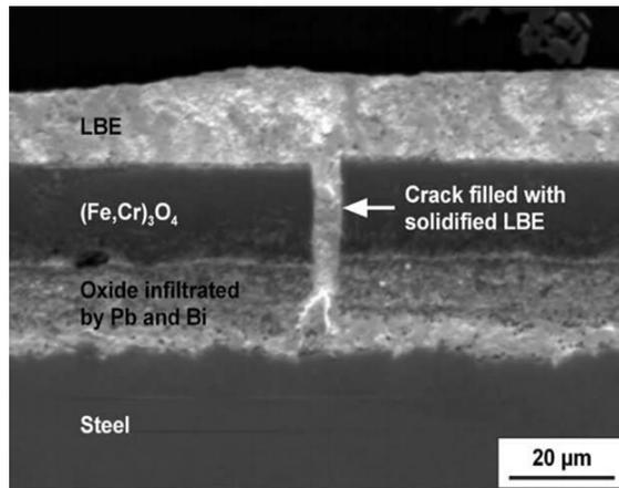
**Fig. 3.11.** SEM<sup>†</sup> image of LBE ingress into the spinel oxide scale on a T91 F/M steel after exposure to flowing LBE at 550 °C for 4015 h ( $v \approx 2$  m/s;  $C_O \approx 1.6 \times 10^{-6}$  wt%) [115].
