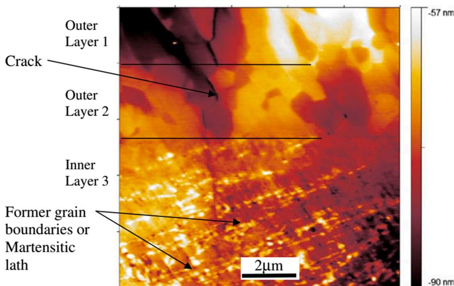
**Fig. 3.12.** AFM<sup>†</sup> image of the complex oxide scales formed on an HT-9 F/M steel exposed to liquid LBE with  $C_O \approx 10^{-6}$  wt% at 550 °C for 3000 h [127].
