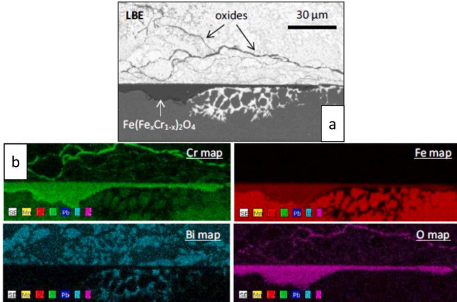
**Fig. 3.7.** EUROFER-97 F/M steel exposed to flowing ( $v \approx 1.8$  m/s) LBE with  $C_O \approx 2.3 \times 10^{-6}$  wt% at 550 °C for 3000 h. The FeCr-spinel oxide scale did not prevent the local occurrence of dissolution corrosion; presumably, a defect in the oxide scale allowed the ingress of LBE, which decorated the oxide/steel interface and attacked intergranularly the steel. (a) SEM<sup>†</sup> image, and (b) EDS<sup>†</sup> maps of the area of interest. Adapted from [92].
