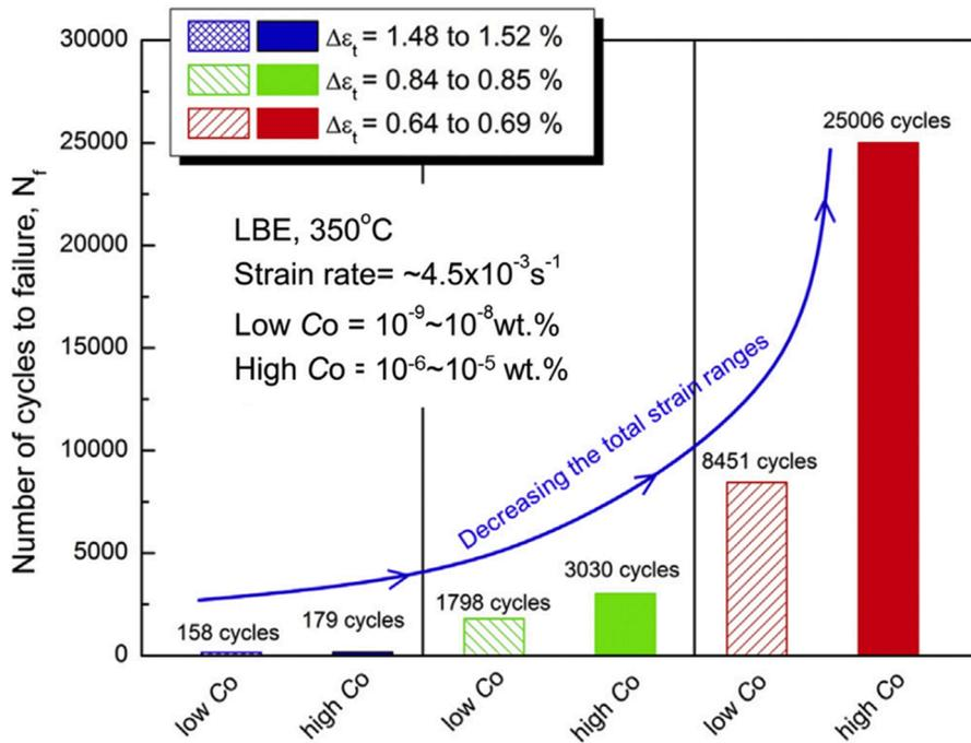
Fig. 4.26. Effect of LBE dissolved oxygen concentration on the fatigue life of T91 F/M steels tested in oxygen-rich ( $C_O \approx 10^{-6}$ – $10^{-5}$  wt%) and oxygen-poor ( $C_O \approx 10^{-9}$ – $10^{-8}$  wt%) liquid LBE at 350 °C, showing that the fatigue life was longer in high-oxygen liquid LBE than in low-oxygen liquid LBE, esp. at relatively low total strain ranges, e.g.,  $\Delta\epsilon_t \approx 0.64$ – $0.69\%$  [537].
