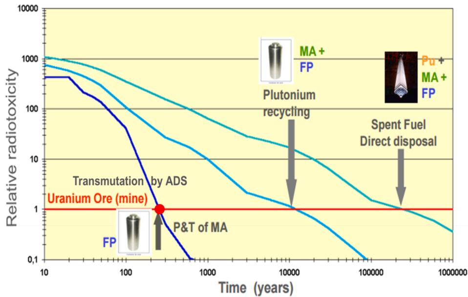
**Fig. 1.1.** Comparison of nuclear waste radiotoxicity before and after transmutation. MA: minor actinides (Am, Np, Cm); FP: fission products; P&T: partitioning & transmutation; Pu: plutonium. Adapted from [17].
