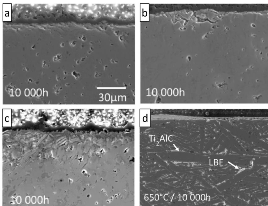
**Fig. 5.8.**  $\text{Ti}_3\text{SiC}_2$  exposed to static liquid LBE ( $C_{\text{O}} \approx 10^{-8}$  wt%) for 10,000 h at (a) 550 °C, (b) 650 °C, and (c) 700 °C. (d)  $\text{Ti}_2\text{AlC}$  exposed to static liquid LBE with  $C_{\text{O}} \approx 10^{-8}$  wt% for 10,000 h at 650 °C. Adapted from [81].
