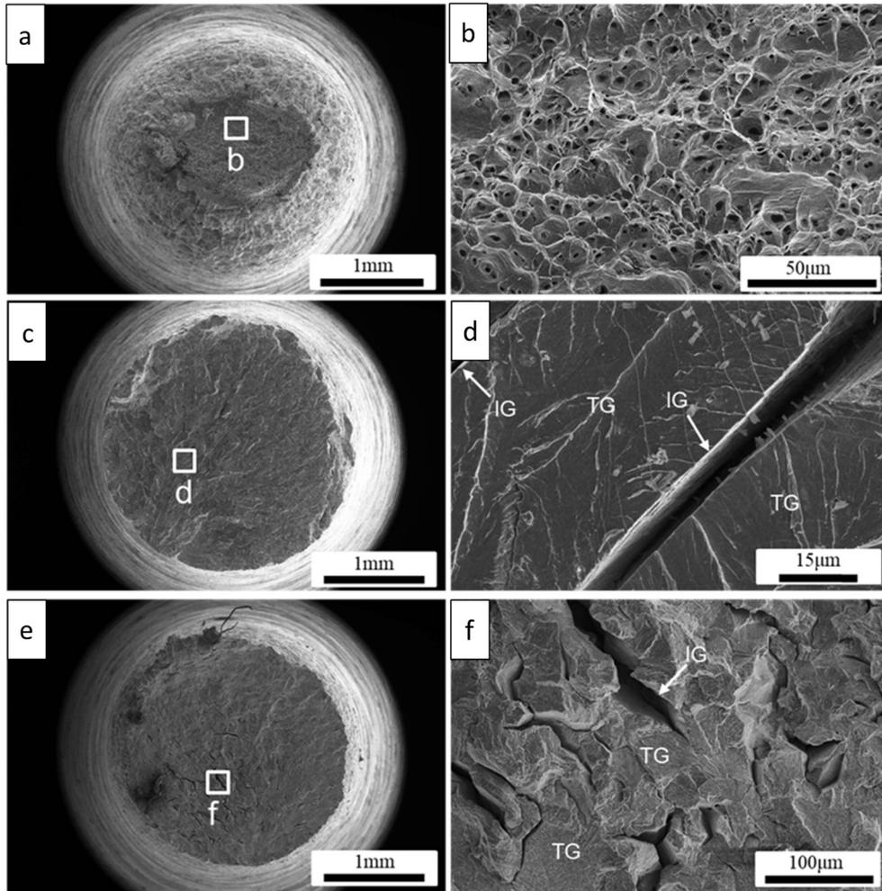
**Fig. 5.4.** SEM<sup>†</sup> images of fracture surfaces of an Fe10Cr4Al alloy tested in tension in Ar (a,b), oxygen-poor (c,d) and oxygen-saturated (e,f) liquid LBE at 350 °C, under an applied strain rate of  $\dot{\epsilon} \approx 5 \times 10^{-4} \text{ s}^{-1}$ . “IG” denotes intergranular cracking; “TG” denotes transgranular cracking. Adapted from [562].
