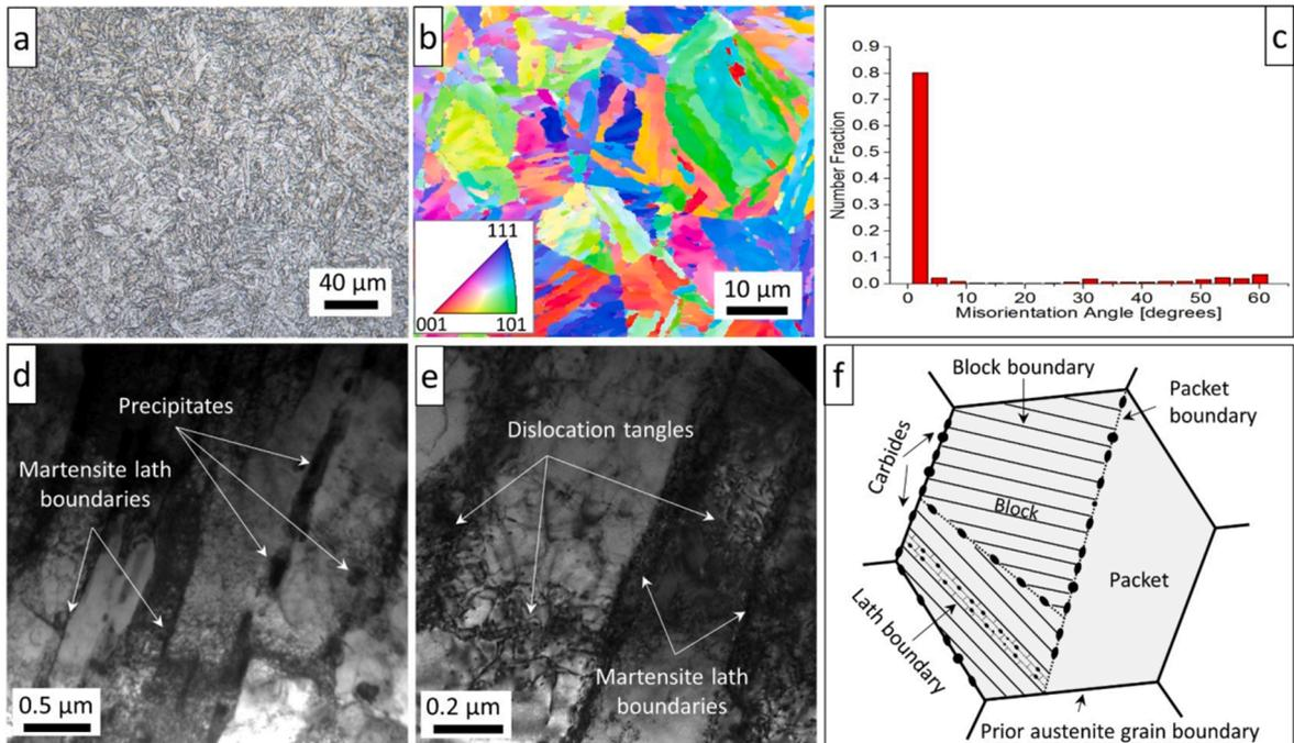
Fig. 2.3. Typical microstructure of a T91 F/M steel: (a) LOM<sup>†</sup> image; (b) EBSD<sup>†</sup> grain orientation map; (c) misorientation angles of martensitic laths; (d, e) TEM<sup>†</sup> bright-field (BF) images; (f) schematic representation of the main microstructural features. Adapted from [53].
