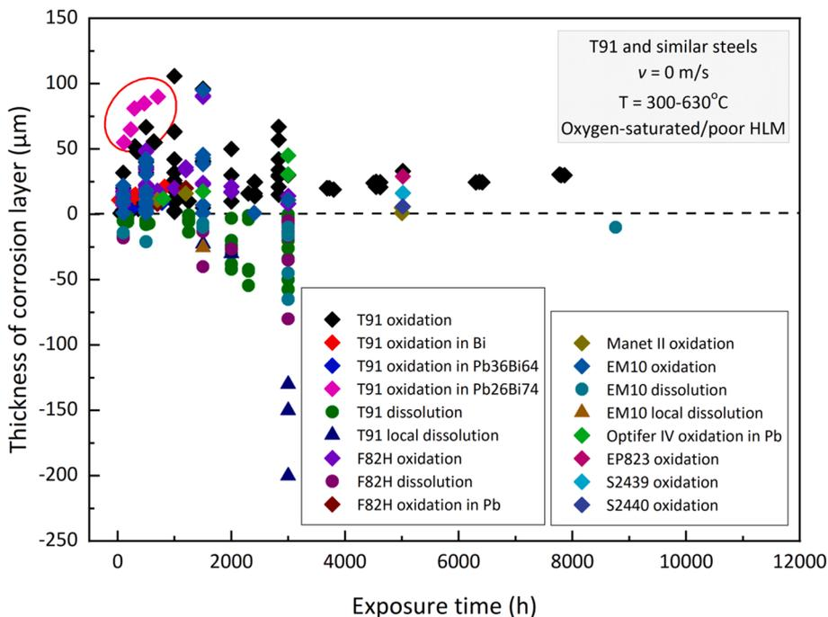
**Fig. 3.33.** Corrosion layer thickness in T91 F/M and similar steels as a function of the exposure duration in *static* HLMs. Steel grades: T91, F82H, Manet II, EM10, Optifer IVc, EP823, S2439 and S2440. HLMs: LBE, Pb, Bi, 36Pb-64Bi and 26Pb-74Bi. Data collected from Refs. [92,116,125,133,136,167,169–171,189,196,198,202–205,208–211,231,233–236]. Mechanisms: uniform oxidation (diamonds), uniform dissolution (circles), locally enhanced dissolution (triangles).
