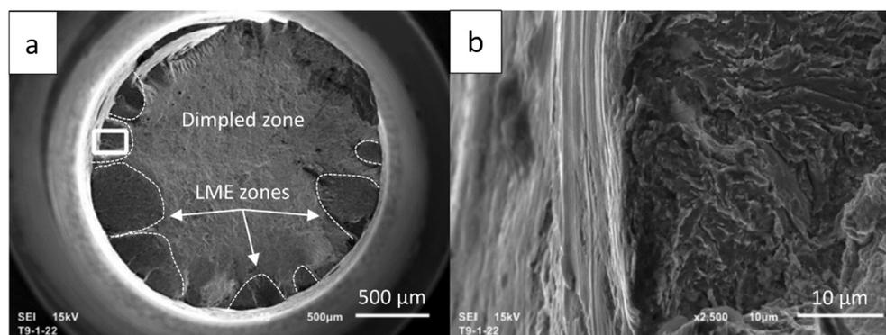
**Fig. 4.33.** SEM<sup>†</sup> images of the fracture surface of T91 F/M steels exposed to static liquid LBE: (a) dimpled zones are observed in the specimen centre and LME-affected zones in its periphery (outlined by white dashed curves), and (b) quasi-cleavage fracture appearance. Test conditions: 350 °C, oxygen-saturated LBE,  $\dot{\epsilon} \approx 5 \times 10^{-5} \text{ s}^{-1}$ . Adapted from [45].
