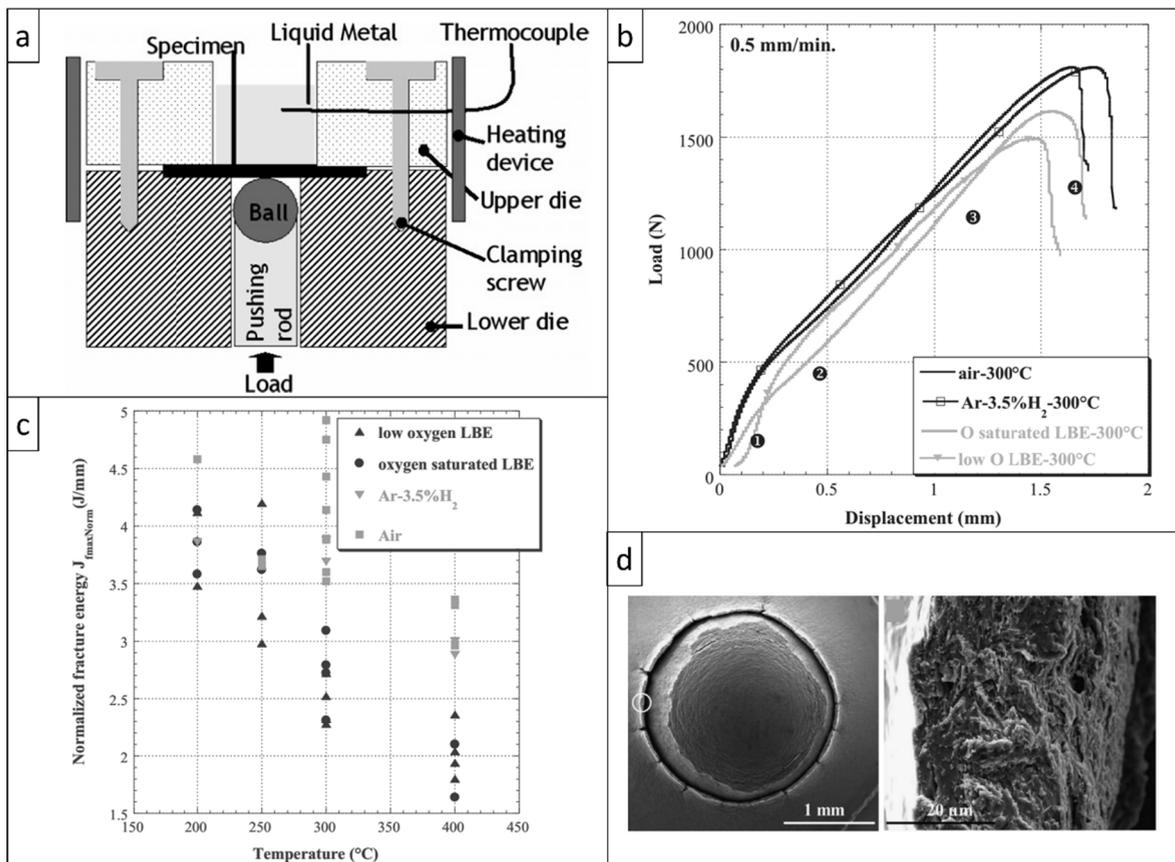
Fig. 4.19. (a) Schematic of an SPT<sup>†</sup> device. (b) Load vs. displacement curves obtained by SPT tests. (c) Fracture energy as a function of test temperature. (d) A typical fracture surface of a disc specimen fractured at 300 °C in liquid LBE upon SPT. Adapted from [504].
