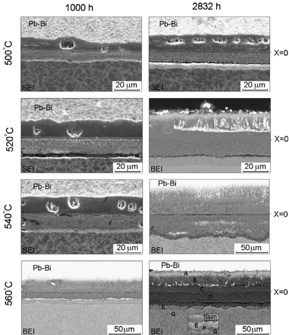
Fig. 3.10. SEM<sup>†</sup> images of oxide scales formed on T91 F/M steels exposed to oxygen-saturated, static LBE at different temperatures (500–560 °C) and for different durations (1000 h, 2832 h). “X = 0” denotes the initial position of the steel surface [125].
