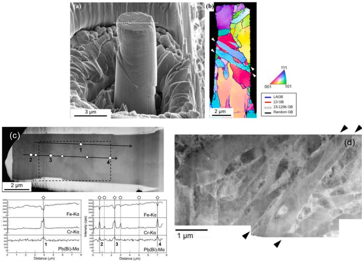
Fig. 4.36. (a) SEM<sup>†</sup> image of a T91 F/M steel micropillar deformed to 9.4% strain, and (b) the corresponding EBSD<sup>†</sup> orientation map with inverse pole figure colour map showing the shear deformation along high-angle GBs marked with arrowheads; (c) EDS<sup>†</sup> point analyses indicating the segregation of LBE segregates at GBs; (d) STEM-HAADF<sup>†</sup> image of the presence of an LBE film at high-angle GBs marked with arrowheads. Adapted from [554].
