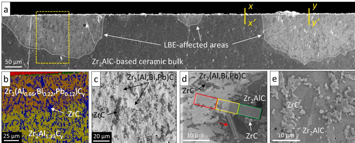
Fig. 5.10. (a) SEM<sup>†</sup> image of the local  $Zr_2AlC/LBE$  interaction, and (b) EDS<sup>†</sup> map of the framed area in (a), showing the formation of a  $Zr_2(Al,Pb,Bi)C$  MAX phase solid solution in the LBE-affected zone. Images of the  $Zr_2AlC/LBE$  interaction: (c) fully affected zone, (d) transition zone, and (e) unaffected sample bulk. Adapted from [648]. Test conditions: 500 °C, 1000 h,  $C_0 \leq 2.2 \times 10^{-10}$  wt%.
