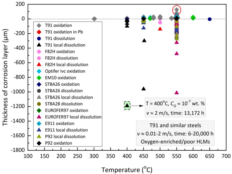
**Fig. 3.29.** Corrosion layer thickness in T91 F/M and similar steels as a function of the exposure temperature in *flowing* HLMs. Steel grades: T91, F82H, Optifer IVc, EM10, STBA26, STBA28, EUROFER-97, E911 and P92. HLMs: LBE, Pb, Bi, 36Pb-64Bi, 26Pb-74Bi. Data collected from Refs. [92,101,115,117,172,180,181,183,185,187,189–191,215–217,219,225,227,230–232,234,237–240]. Mechanisms: uniform oxidation (diamonds), uniform dissolution (circles), and locally enhanced dissolution (triangles).
