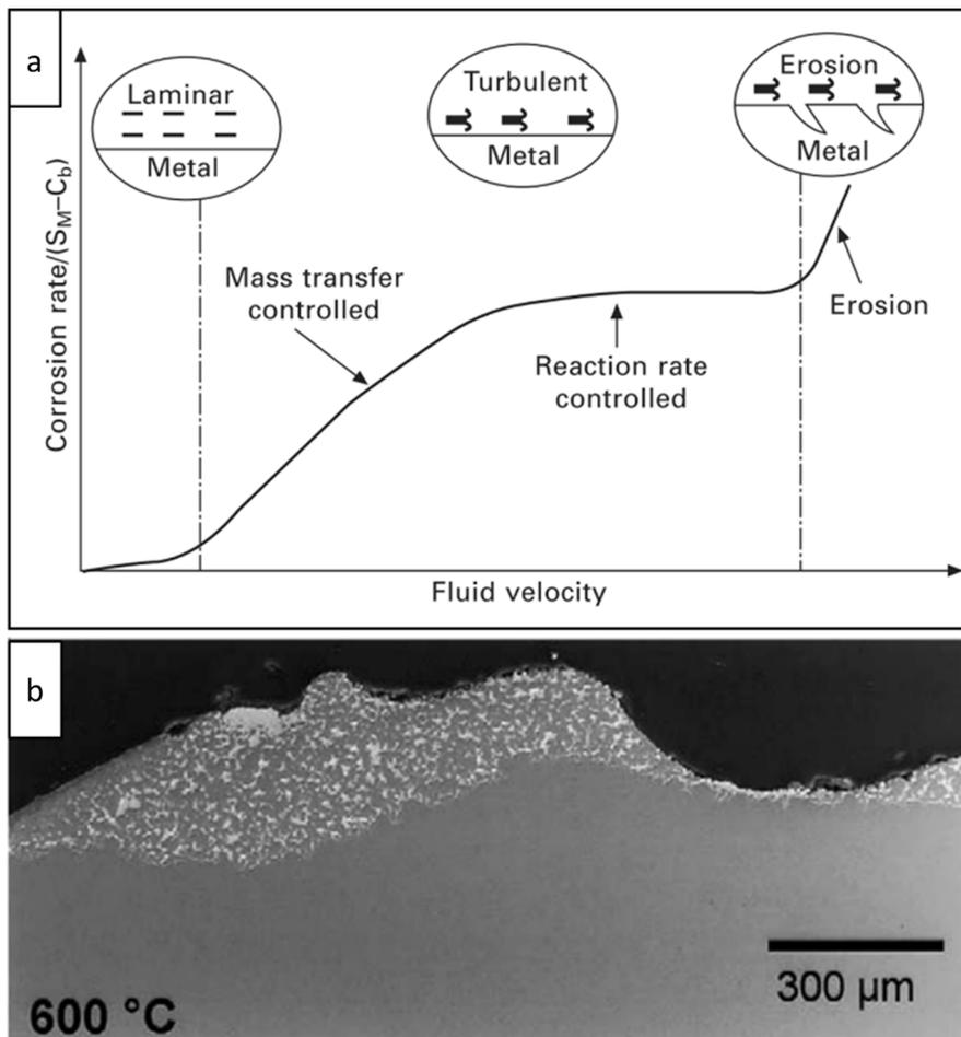
Fig. 3.5. (a) Corrosion mechanisms as a function of the HLM flow velocity [103]; (b) SEM<sup>†</sup> image of material losses caused by erosion/corrosion in 316L AuSS exposed to flowing LBE ( $v \approx 2$  m/s,  $C_O \approx 10^{-6}$  wt%) at 600 °C for 2000 h. Adapted from [104].
