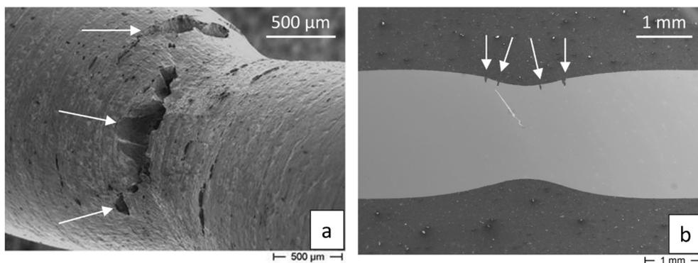
**Fig. 4.32.** SEM<sup>†</sup> images of the localisation of LME-induced microcracks (arrows) in the ‘neck’ area of T91 F/M steel specimens tested in tension in static liquid LBE. Test conditions: 350 °C,  $\dot{\epsilon} \approx 5 \times 10^{-5} \text{ s}^{-1}$ ,  $C_{\text{O}} \approx 10^{-10}$ – $10^{-9}$  wt%. (Unpublished data produced by the authors).
