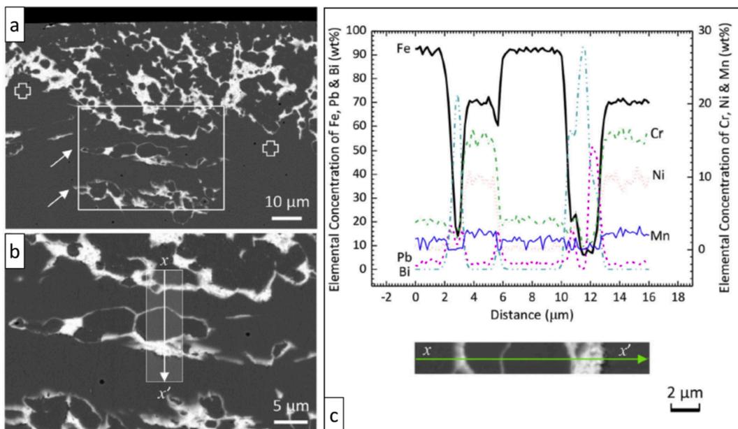
**Fig. 3.20.** CW 316L AuSS exposed to oxygen-poor ( $C_O < 2 \times 10^{-8}$  wt%), static LBE at 500 °C for 3282 h. (a,b) SEM<sup>†</sup> images of groups of grains ahead of the main dissolution front (crosses), which underwent selective leaching during steel exposure. (c) The EDS<sup>†</sup> line scan shows selective leaching of Ni, Mn and Cr; Fe enrichment; and Pb/Bi presence at GBs. Adapted from [40].
