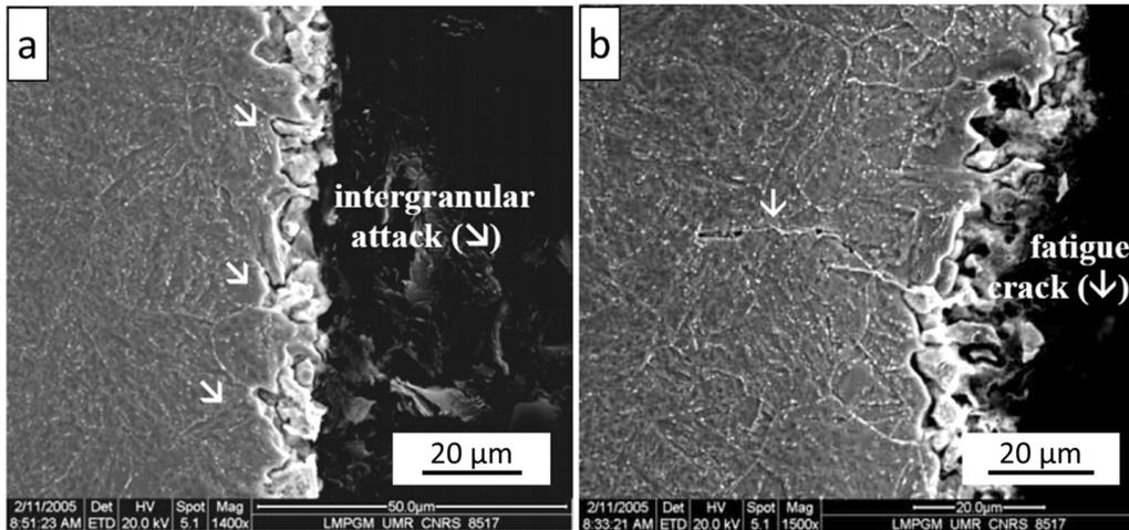
Fig. 4.29. SEM<sup>†</sup> images of T91 F/M steels after pre-exposure to oxygen-poor ( $C_O < 10^{-10}$  wt%) liquid LBE at 600 °C for 613 h: (a) before fatigue testing, (b) after fatigue rupture in liquid LBE at 300 °C and  $\Delta\epsilon_t = 2.2\%$ . Adapted from [231,495,540].
