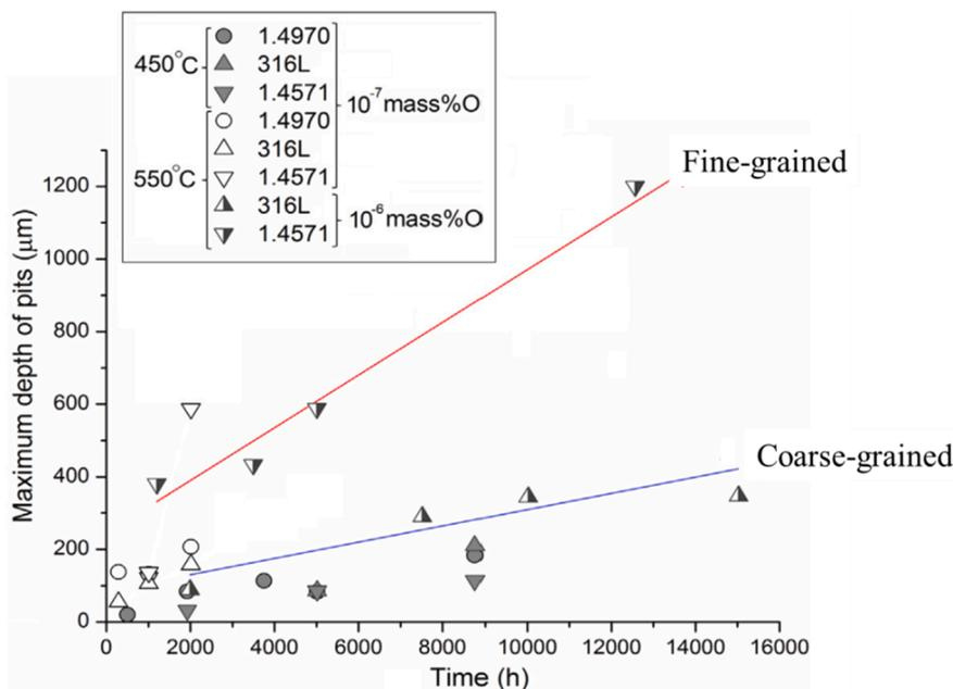
Fig. 3.23. Maximum ‘pit’ depths observed in 316L, 1.4970 and 1.4571 AuSS exposed to flowing LBE ( $v \approx 2$  m/s) under different exposure durations, oxygen concentrations, and temperatures. Adapted from [43].
