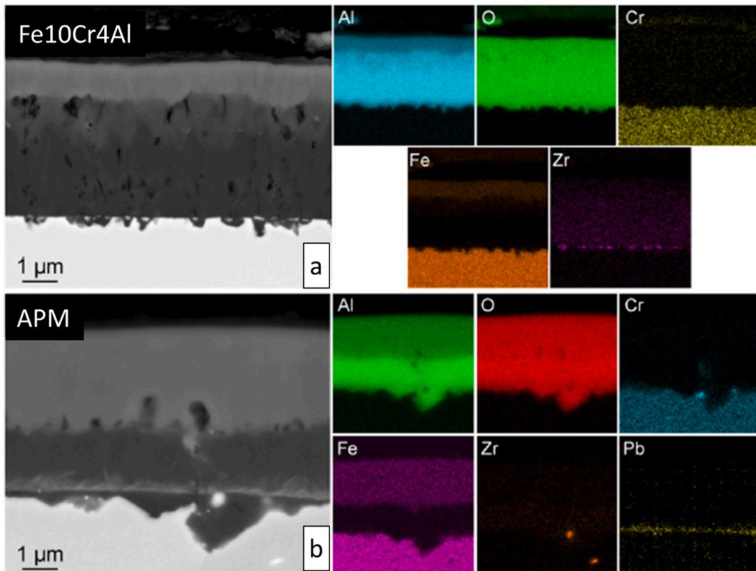
**Fig. 5.3.** EDS<sup>†</sup> elemental maps of (a) Fe10Cr4Al and (b) APM (Fe21Cr5.8Al) alloys after exposure to liquid Pb at 800 °C, showing the formation of an Fe-enriched Al<sub>2</sub>O<sub>3</sub> scale. Adapted from [618]. In this case, Fe10Cr4Al was proposed as a candidate structural material for concentrated solar power (CSP) systems, which require high operation temperatures for better thermal efficiency.
