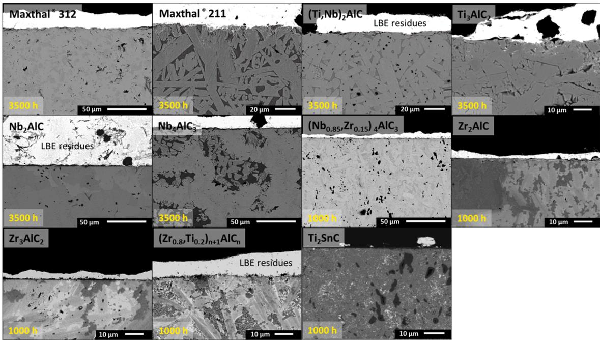
Fig. 5.9. SEM<sup>†</sup> images of the interaction between various MAX phase ceramics and static liquid LBE; exposure conditions: 500 °C, 1000–3500 h,  $C_0 \leq 2.2 \times 10^{-10}$  wt% [83].
