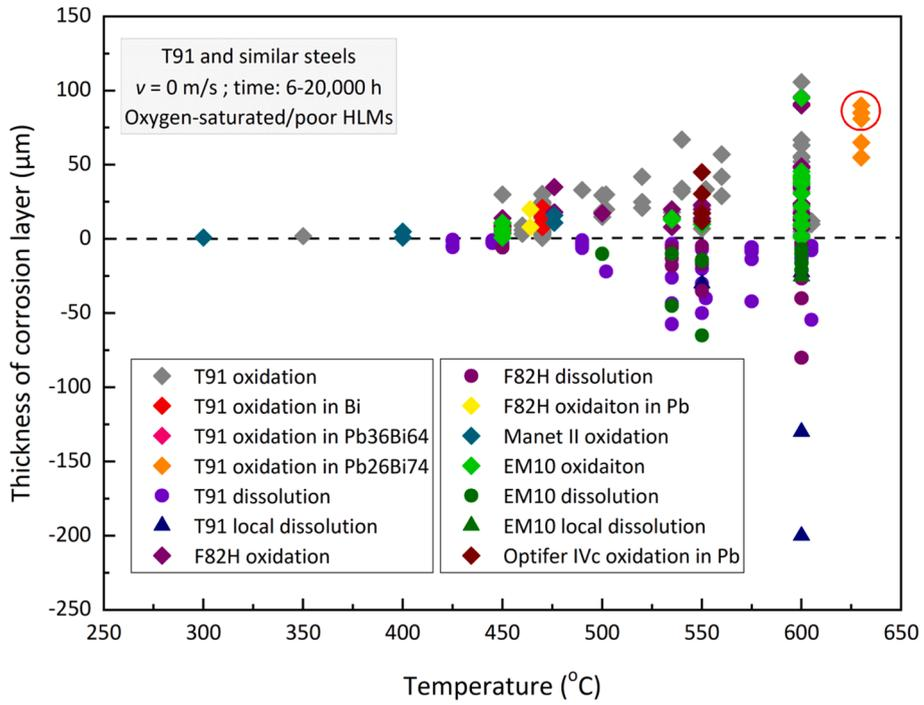
**Fig. 3.28.** Corrosion layer thickness in T91 F/M and similar steels as a function of the exposure temperature in *static* HLMs. Steel grades: T91, F82H, Manet II, EM10 and Optifer IVc. HLMs: LBE, Pb, Bi, 36Pb-64Bi, 26Pb-74Bi. Data collected from Refs. [92,116,125,133,136,167,169–171,189,196,198,202–205,208–211,231,233–236]. Mechanisms: uniform oxidation (diamonds), uniform dissolution (circles), and locally enhanced dissolution (triangles).
