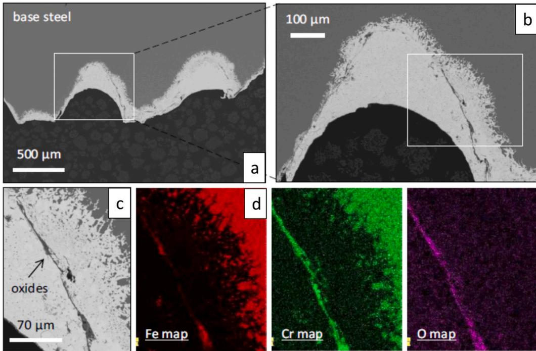
**Fig. 3.6.** Enhanced local LBE dissolution attack in an ODS-EUROFER-97 ferritic steel exposed to flowing ( $v \approx 2$  m/s) LBE with  $C_O \approx 1.4\text{--}1.6 \times 10^{-6}$  wt% at 550 °C for 5012 h. LBE dissolution attack occurs in the narrow space ('crevice') between the screw threads connecting two cylindrical specimens with each other. (a-c) SEM<sup>†</sup> images, and (d) EDS<sup>†</sup> maps of areas of interest. Adapted from [92].
