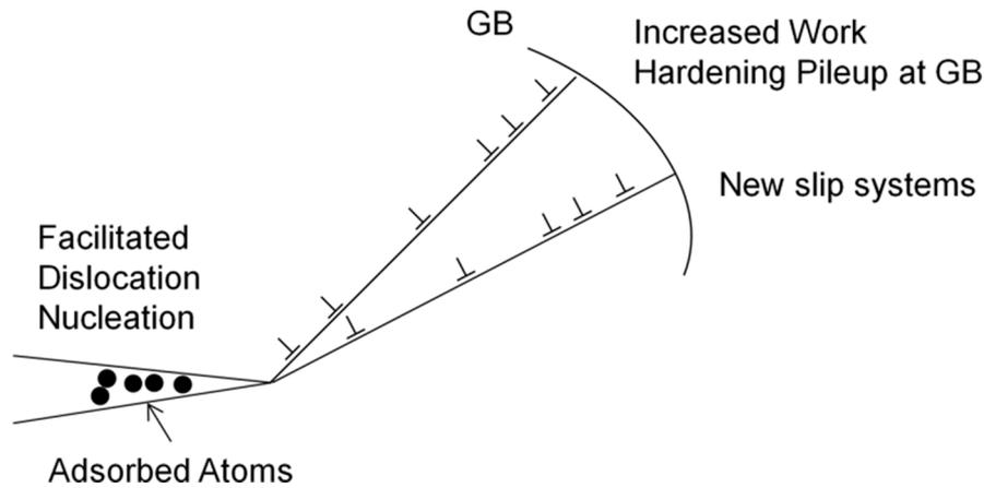
**Fig. 4.12.** Schematic illustration of the enhanced work hardening model, whereby the greatly enhanced emission of dislocations (effectively leading to the local crack tip work hardening) facilitated by the adsorbed liquid metal atoms increases significantly the crack growth rate.
