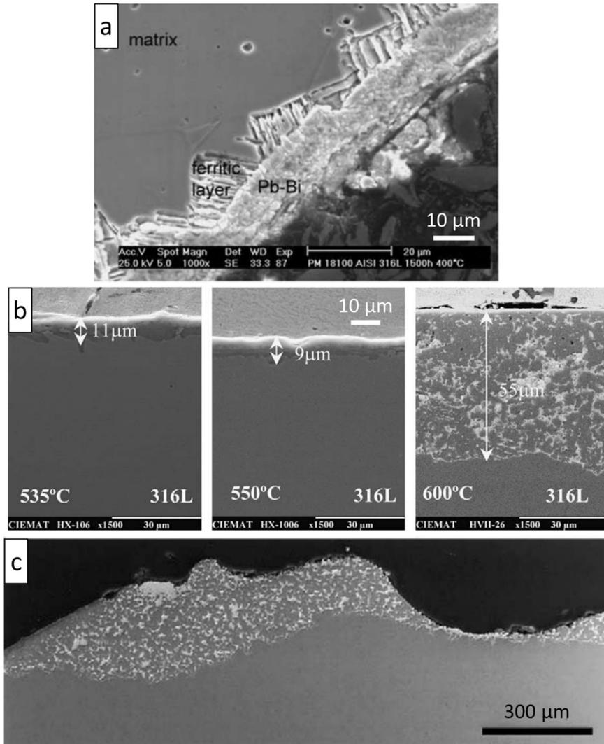
**Fig. 3.21.** SEM<sup>†</sup> images of surface ferritisation in 316L AuSS exposed to liquid LBE. Test conditions: (a) 400 °C, 1500 h, flowing LBE ( $v \approx 1$  m/s),  $C_O \approx 10^{-10}$ – $10^{-8}$  wt%; (b) 500 h, 535/550/600 °C, static LBE,  $C_O \approx 3$ – $8 \times 10^{-6}$  wt%; (c) 600 °C, 2000 h, flowing LBE ( $v \approx 2$  m/s),  $C_O \approx 1 \times 10^{-6}$  wt%. Adapted from [104,136,180].
