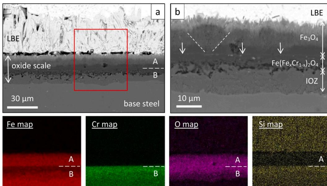
Fig. 3.1. SEM<sup>†</sup> images of the complex oxide scale on Si-doped EP-823 F/M steel exposed to oxygen-rich, static LBE at 490 °C for 5016 h. The oxide scale consists of magnetite ( $\text{Fe}_3\text{O}_4$ ; area A), FeCr-spinel ( $\text{Fe}(\text{Fe}_x\text{Cr}_{1-x})_2\text{O}_4$ ) & IOZ<sup>†</sup> (area B). EDS<sup>†</sup> maps show no Si in magnetite. This oxide scale shows fine porosity at the FeCr-spinel/IOZ interface. Adapted from [92].
