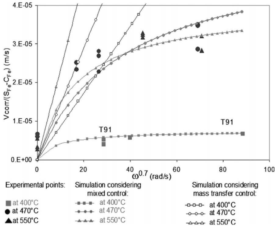
Fig. 3.22. Ratio between the dissolution corrosion rate,  $V_{corr}$ , and the  $(S_{Fe}-C_{Fe})$  factor as a function of the steel specimen angular velocity,  $\omega$ , at 400, 470, and 540 °C [185].
