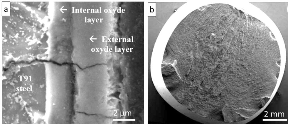
**Fig. 4.30.** SEM<sup>†</sup> images of T91 F/M steels after pre-exposure to oxygen-saturated liquid LBE at 470 °C for 502 h and fatigue testing in liquid LBE at 300 °C and  $\Delta\epsilon_t = 0.4\%$ . Cross-section (a) and fracture surface (b). Adapted from [231,495,540].
